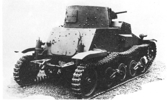
Three views (three-quarter left front, three-quarter right rear, and rear) of the Improved Type 94 Tankette built by the Tokyo Gas and Electric Industry in 1936. In the rear views note the perpendicular cylinder enclosing a coil spring by means of which the rear idler bore the weight of the aft portion of the chassis. A Type 94 37mm Gun is mounted in this version.
