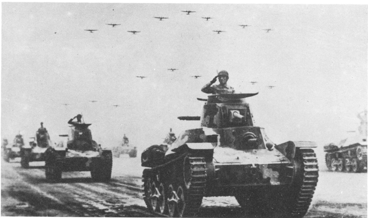
Type 95 Light Tanks marching past. Note the turret machine-gun in the five o'clock position.
