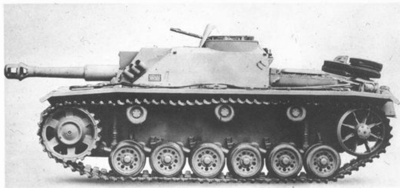
10,5cm Sturmhaubitze 42 Ausf. G, SdKfz 142/2 or Sturmgeschuetz III mit 10,5cm StuH 42 L/28 3 or StuG III fuer 10,5cm StuH 42 This equipment with respect to the chassis and superstructure was identical to the Sturmgeschuetz 40, but it was armed with the 10,5cm Sturmhaubitze 42 L/28 (Assault Howitzer) that had been adapted to this role. Late production models had no muzzle brakes and were fitted with remote-controlled machine guns on the roof. Some vehicles in this series were fitted with a modified version of the cast gun mantlet Saukopf. Crew 4. Weight 24 tons.
