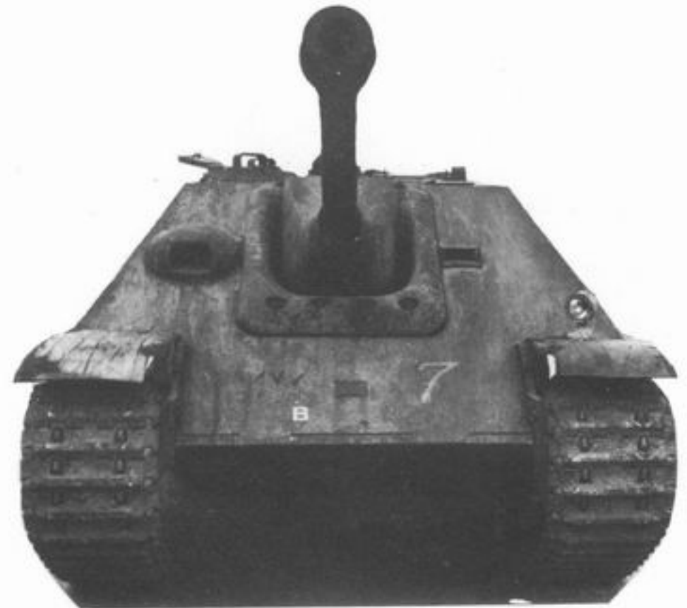
Jagdpanther with heavy bolted gun mantlet.
