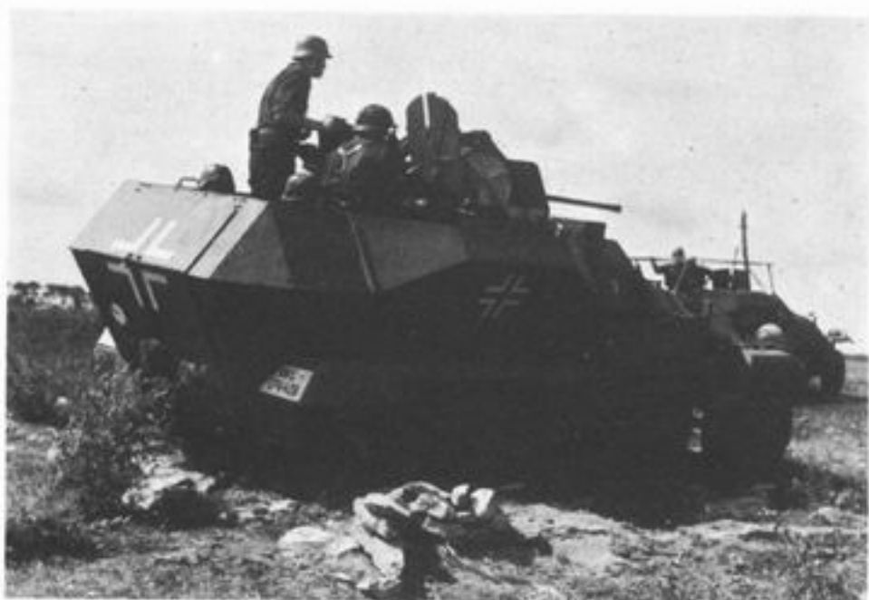
Luftwaffe, mSchtzPzWg (2cm Flak 38) Developed for the Luftwaffe Flak troops, several were built and tested in troop trials. This equipment consisted of the 2cm Flak 38 on a modified SdKfz 251. To allow the gun to be installed in the fighting compartment, the body was redesigned so that the sides of the vehicle could be folded down to allow full traverse of the gun. (Bundesarchiv, Koblenz)
