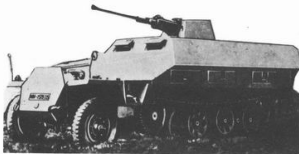
mSchtzPzWg mit 2cm Flak 38 SdKfz 251/17 Developed as a flak vehicle in 1944, and built in limited numbers this series became standard equipment. The gun, in a small armoured turret, was positioned behind the driver's compartment with the gun barrel projecting over the armoured cab of an SdKfz 251. Crew 4/6.
