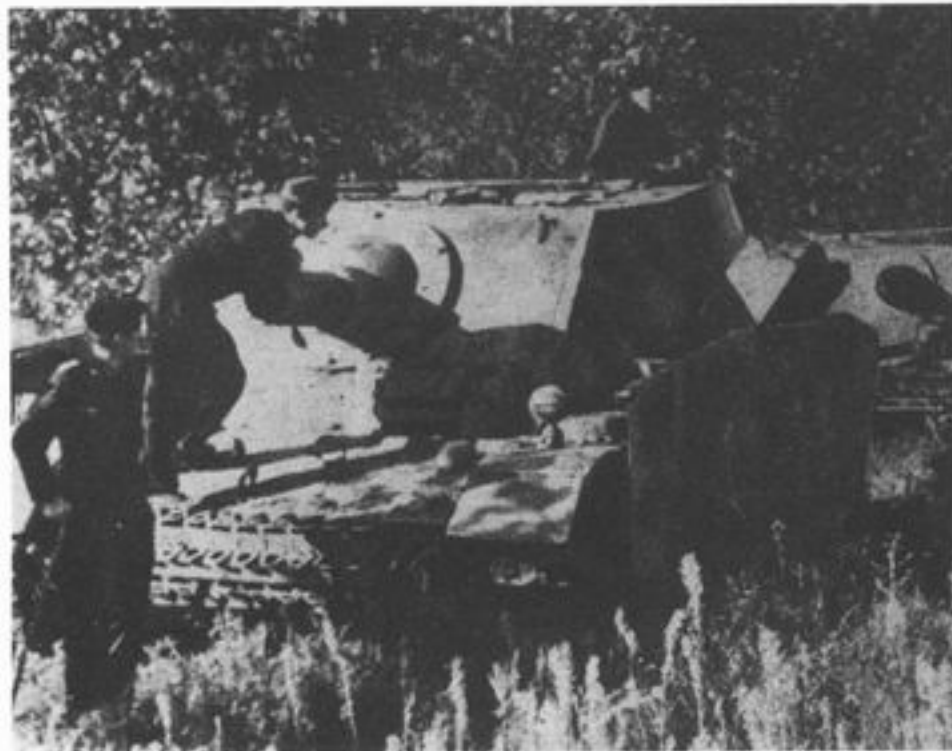
10.5cm Sturmhaubitze 42 Ausf. G without muzzle brake. Equipped with armour skirting.
