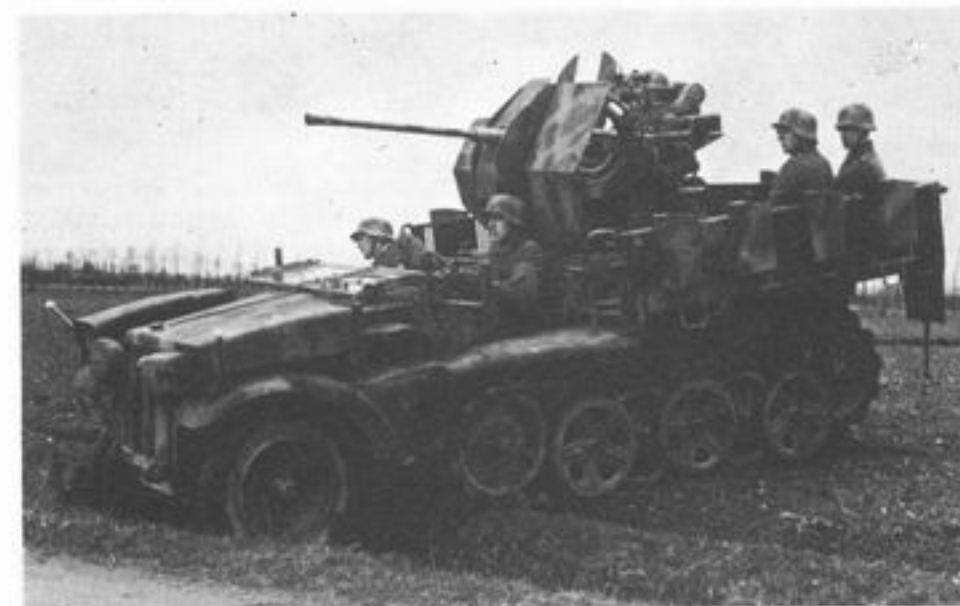
Leichte Selbstfahrlafette (2cm Flak 30) SdKfz 10/4 2cm Flak gun mounted on 1-ton semi-tracked vehicle SdKfz 10. The sides of the vehicle were dropped when in action to facilitate all round traverse. Spare ammunition was carried in a towed two-wheeled limber. Crew 7. Weight 5.5 tons. (Bundesarchiv, Koblenz)
