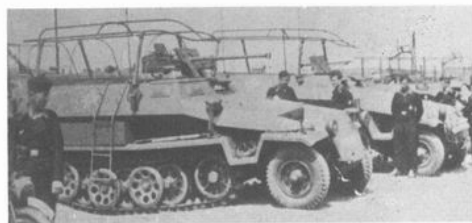
Medium personnel carrier SdKfz 251 equipped with the 2,8cm anti-tank gun. This was not a standard fitting on this class of vehicle.
