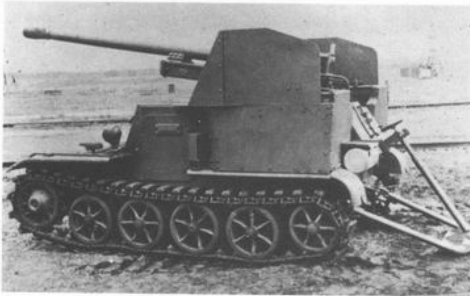
Borgward PzSfl Ia fuer 5cm Pak 38 L/60 Based on the Borgward ammunition carrier VK 301, two prototypes were converted to mount the 5cm Pak 38 during 1940. Project dropped.
