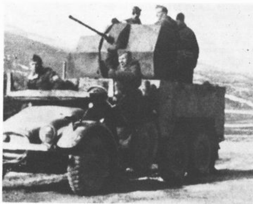
2cm Flak 38 auf le gl Lkw Kfz 70 This was a standard conversion, and consisted of the 2cm Flak gun carried in the rear compartment of a 6 × 4 light truck, (Type Krupp L2H143) used by the Luftwaffe.
