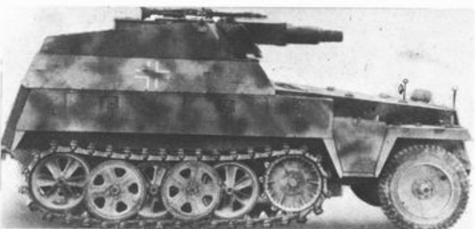
Leichter Schuetzenpanzerwagen mit 7,5cm KwK L/24 SdKfz 250/8 Light Personnel Carrier SdKfz 250 equipped with the short 7,5cm gun in new mounting. An MG 42 machine gun was mounted on the gun to give co-axial fire and also to act as a ranging gun for the latter. Crew 3. Weight 6 tons.
