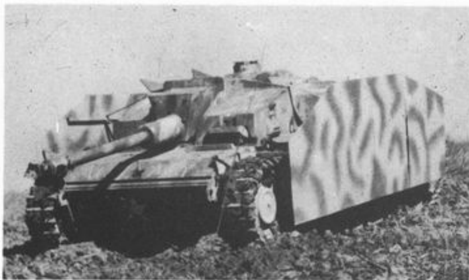
7,5cm Sturmgeschuetz 40 Ausf. F/8 Only a small series of the StuG III Ausf. F were armed with the L/43 gun. The Ausf. F/8 was then fitted with a longer gun, the 7,5cm Sturmkanone (StuK) 40 L/48.
