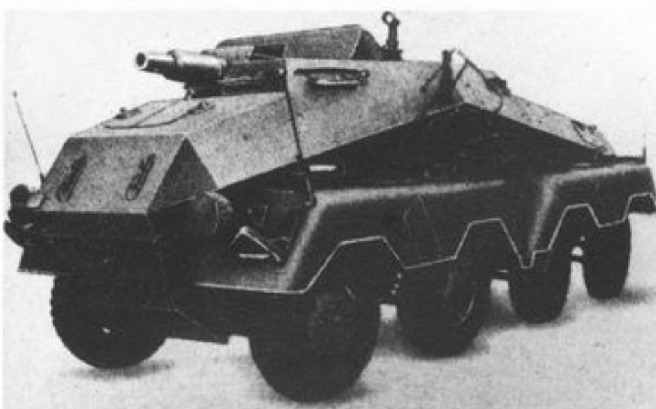
Panzerspähwagen (SdKfz 233) mit 7,5cm StuK L/24 or Schwerer Panzerspähwagen (sPzSpWg) (7,5cm L/24) SdKfz 233, 8-Rad Heavy eight-wheeled armoured car SdKfz 233 with early cut-away gun mounting. Crew 3. Weight 7.55 tons.
