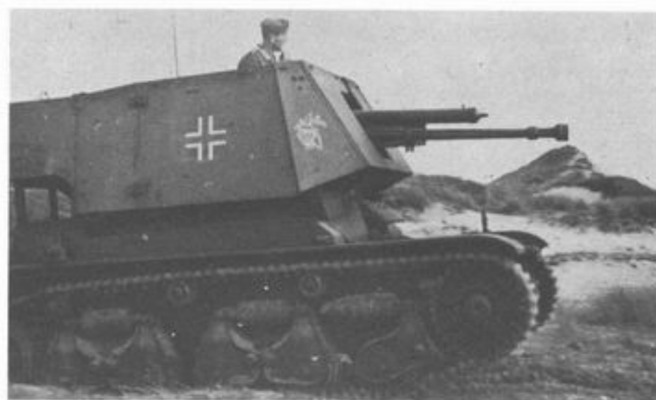
Top left 4,7cm Pak 181 oder 183(f) auf PzJaeg Lorraine Schlepper (f) Produced in limited numbers during 1941, this equipment consisted of the unmodified French Lorraine Tracteur Blindé 38L with either the French 47mm M/E 1937 or M/E 1939 anti-tank gun mounted on a pedestal at the rear of the vehicle. Crew 3. Weight 6 tons.
