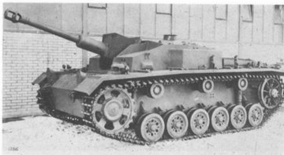
7,5cm Sturmgeschuetz 40, Ausf. F SdKfz 142/1 or Sturmgeschuetz III Ausf. F Early in 1942 the first StuG models with a long barrel 7,5cm StuK 40 L/43 were introduced. This was a development of the KwK 40 tank gun adapted for use in the assault type of vehicle. Based on a chassis similar to that of the StuG III Ausf. E, this vehicle had a modified superstructure fitted with an electric fan on top to ventilate the fighting compartment. Crew 4. Weight 21.6 tons.
