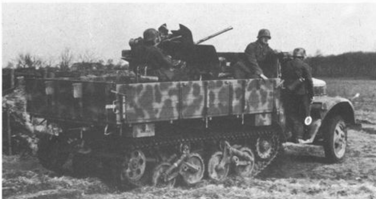
3,7cm Flak 36 auf Maultier This equipment consisted of the 3,7cm Flak gun mounted on a Ford 2-ton semi-tracked cargo vehicle. (Gleisketten-Lkw, 2t (Maultier) ) (Bundesarchiv, Koblenz)
