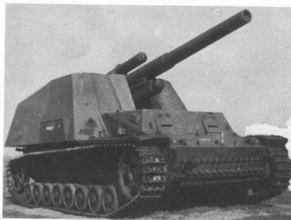
A late production Hummel with the redesigned front superstructure. (Warpics)
