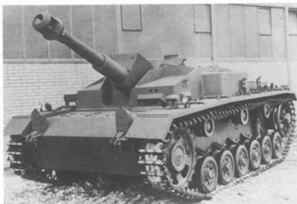
10,5cm Feldhaubitze 42 SdKfz 142/2 or Sturmhaubitze 42 Ausf. F With the adoption of the long L/43 7,5cm gun in place of the short 7,5cm low velocity gun on the StuG III models there remained a limited requirement for howitzer-armed vehicles for the close support role. As developed, this close support weapon had the usual characteristics of the StuG but was confined to a purely anti-personnel role, firing high explosive and not armour-piercing ammunition as did the up-gunned StuG models. Produced in 1942, the first of the assault howitzer vehicles were armed with the 10,5cm 1e FH 18, a light field howitzer adapted for use in the StuG. Identical to Sturmgeschuetz 40 Ausf. F, only a few of these vehicles were built. Crew 4. Weight 23 tons.
