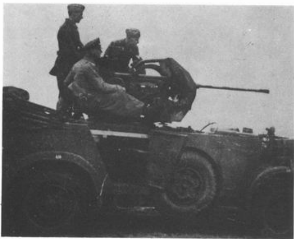
2cm Flak 38 auf Mannschaftskraftwagen 2cm anti-aircraft gun model 38 in the rear compartment of an Auto-Union 4 × 4 personnel car. The weapon was mounted on a raised platform.
