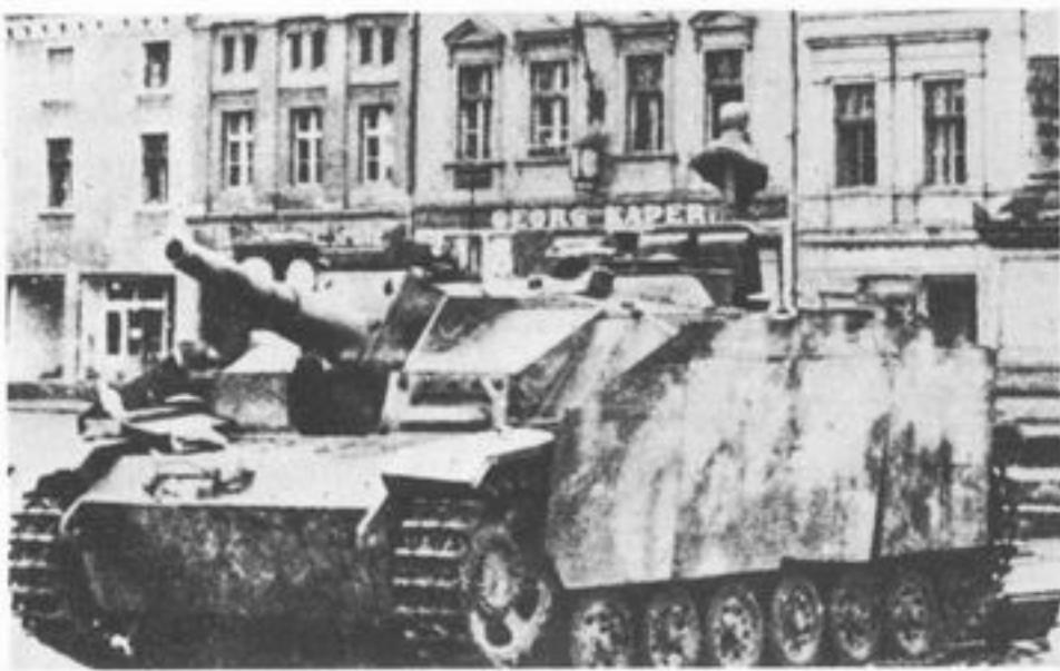
10.5cm Sturmhaubitze 42 Ausf. G without muzzle brake. Equipped with armour skirting.
