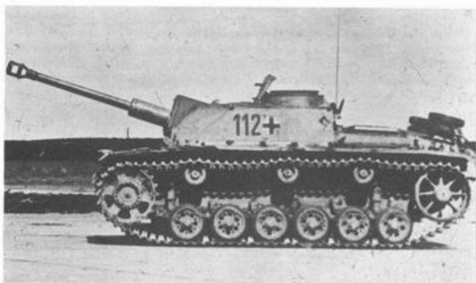
7,5cm Sturmgeschuetz 40 Ausf. G SdKfz 142/1 or StuG III Ausf. G fuer StuK 40 L/48 This model appeared at the end of 1942 and was based on the Panzerkampfwagen III Ausf. J. Again various changes had taken place. The longer gun, the Sturmkanone 40, was fitted and the nose frontal armour increased. The roof of the superstructure was equipped with a circular commander's cupola, with seven episcopes—previously the commander had had a fixed hatch through which the artillery scissors periscope projected. Also on the roof was a small armour shield for use with the machine gun. Later vehicles were fitted with armoured skirting and treated with Zimmerit (Anti-magnetic grenade plaster). Crew 4. Weight 23.9 tons.
