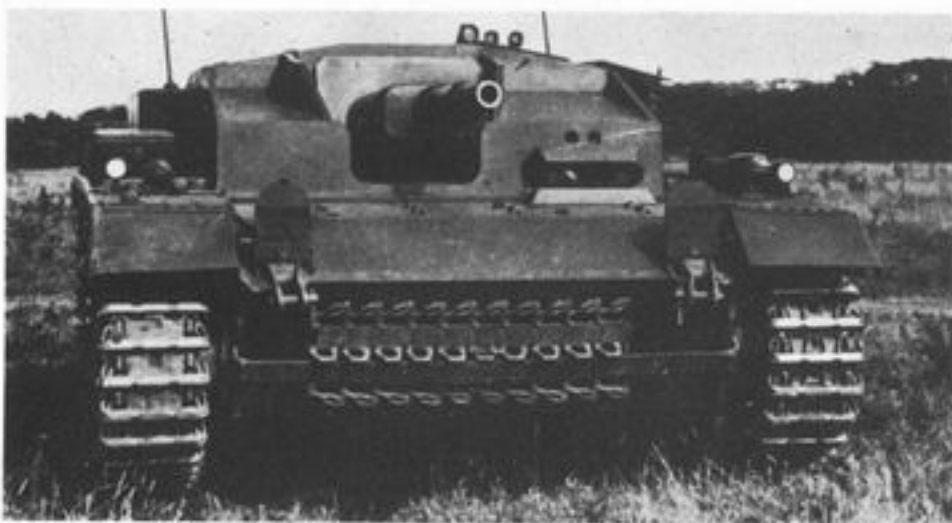
Sturmgeschuetz III, Ausf. E SdKfz 142 Produced in 1942, this was the last model to be armed with the short barrellled 7,5cm KwK L/24. Though similar to the previous models, this vehicle was fitted with an additional armoured pannier on the right side to carry extra radio equipment when in use as a Zugführerwagen (Unit Commander's vehicle).
