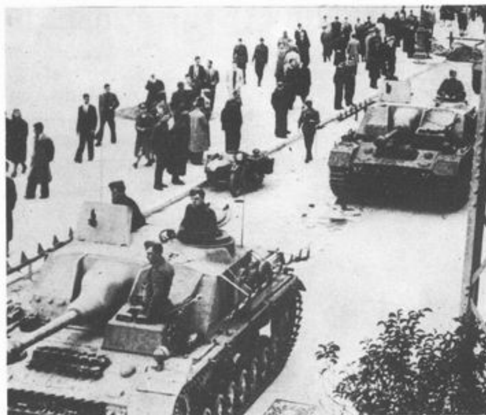
Sturmgeschuetz IV L/48 (7,5cm StuK 40) SdKfz 163 or StuG IV fuer 7,5cm StuK 40 Produced from 1943, this equipment consisted of the 7,5cm StuK 40 mounted on the chassis of the Panzerkampfwagen IV Ausf. H or J. The superstructure was modified from that of the StuG III Ausf. G, late model with Saukopf mantlet. Armour protecting was increased by the addition of slabs of concrete six inches thick attached to the front plate and roof over the driver's compartment. Late models were equipped with a remote-controlled machine gun on the roof. Crew 4. Weight 23 tons.
