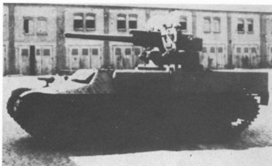
4,7cm Pak (t) Sfl auf PzKpfw I Ausf. B or Panzerjaeger I fuer 4,7cm Pak (t) Introduced into service in 1940, this was the first self-propelled anti-tank gun to enter German service. Based on the chassis of the Panzerkampfwagen I Ausf. B, this equipment was fitted with a Czech 4,7cm anti-tank gun L/43 mounted within a three-sided gun shield. Crew 3. Weight 6 tons.
