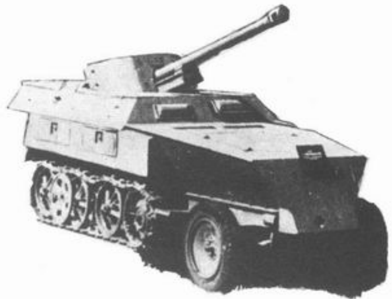
5cm Pak 38 auf leichter Schuetzenpanzerwagen SdKfz 250 5cm Pak mounted on the light semi-tracked personnel carrier SdKfz 250. Nothing known, believed to be a trials vehicle.
