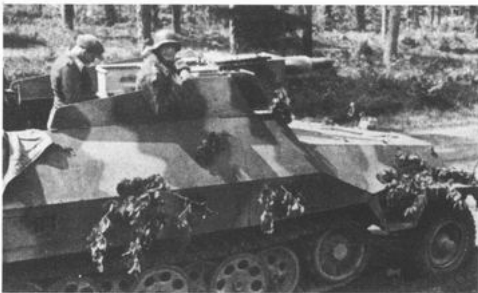
Mittlerer Schuetzenpanzerwagen (7,5cm KwK L/24) SdKfz 251/9 Armoured Personnel Carrier SdKfz 251 with 7,5cm KwK L/24 in the early recessed gun mounting. Crew 3. Weight 8.53 tons.
