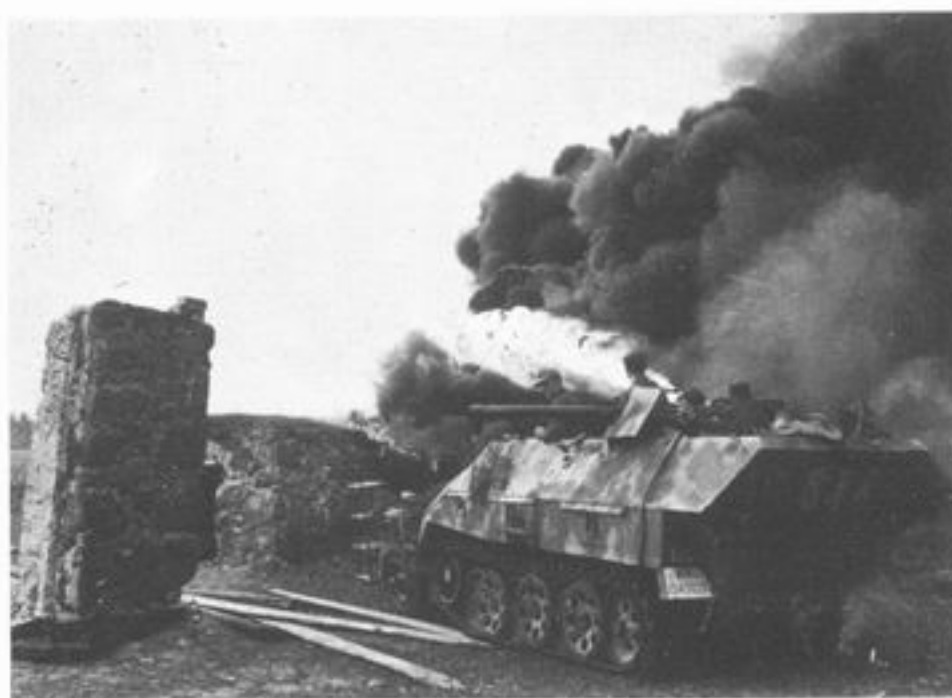
This view shows the 1.4cm projector on the right side of the vehicle in action against a target. This vehicle is a late production model without the portable equipment. (Bundesarchiv, Koblenz)
