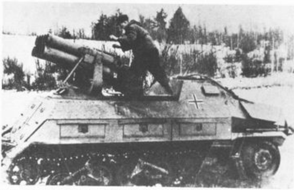
15cm Panzerwerfer 42 auf 'Maultier' (Opel) SdKfz 4/1 Rocket projectors were introduced in 1940 for laying heavy concentrations of smoke and high explosive on target areas, the original 15cm 6-barrel projector equipment being mounted on a two-wheeled towed carriage. To increase the mobility and rate of fire of this weapon, ten projector tubes were mounted on a converted semi-tracked cargo vehicle. The mobile mount used for this conversion was the 2-ton Opel 3.6.36 Type S/SSM that had been fitted with a light armoured body. The projectors in two horizontal rows of five were mounted at the rear of the vehicle on a turntable with a 360 degree traverse. An additional ten 15cm rocket rounds were carried inside the vehicle. Crew 3. Weight 7.1 tons.
