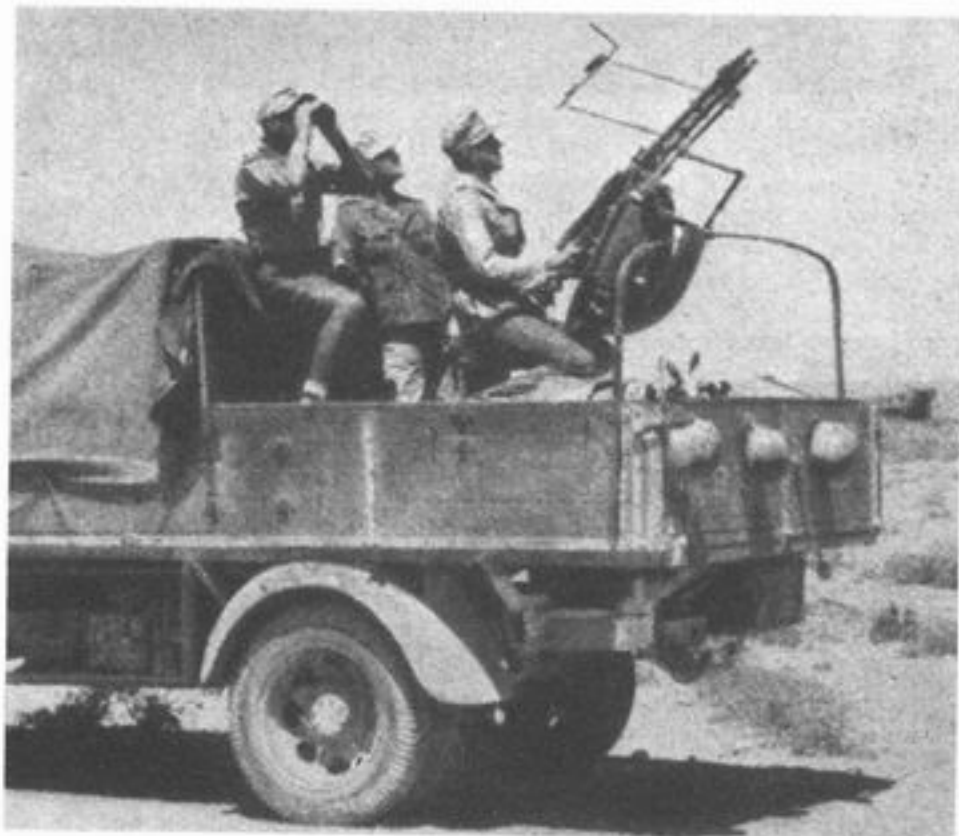
The Zwillingslafette 36 was a universal MG mount that could be adapted to fit most vehicles, including rail-wagons. The picture shows the mount on a medium type truck.
