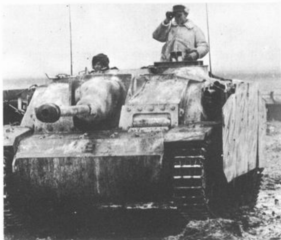
7,5cm Sturmgeschuetz 40 Ausf. G (Saukopf) SdKfz 142/1 This was the final production version of the Sturmgeschuetz III and was similar to the Ausf. G, but it had heavier armour and a cast gun mantlet called a Saukopfblende or Saukopf (Pig's Head). Final production vehicles were equipped with a remote controlled machine gun on the turret roof. Crew 4. Weight 24.5 tons. (Bundesarchiv, Koblenz)
