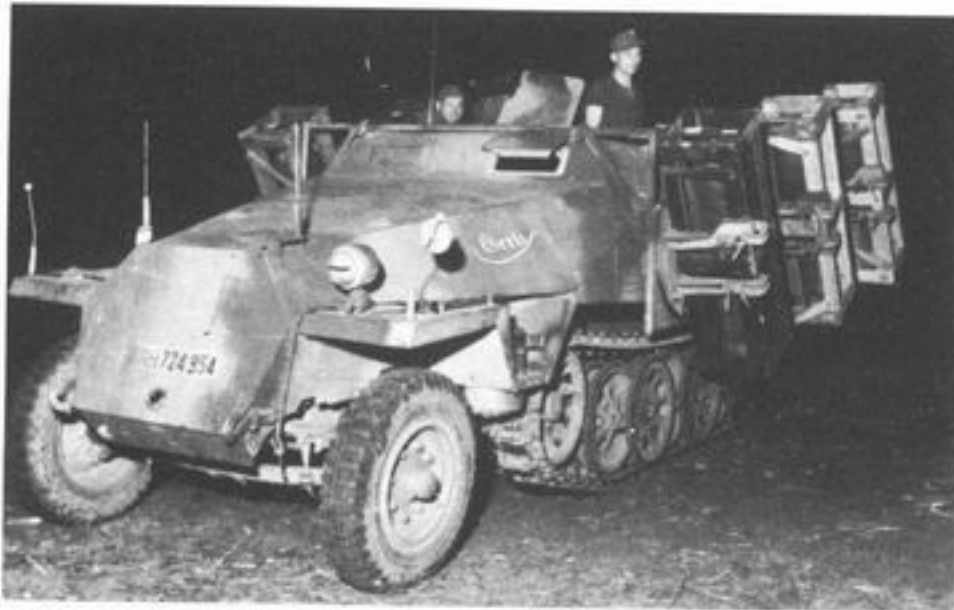
Mittlerer Schuetzenpanzerwagen mit Wurffrahmen, SdKfz 251/1 Introduced into service during 1940, this equipment consisted of the standard 3-ton semi-tracked personnel carrier SdKfz 251 equipped with externally mounted pivoting racks for launching the heavy 28 or 32cm rockets. The racks known as the Schweres Wurffrahmen 40 (SWR 40) were attached, three on each side of the vehicle, and were designed to fire the rocket from the crate that it was packed in, thereby utilising the crate as the projector. The pivoting plates within the SWR 40 frames or racks were adjustable for elevations from 5 to 45 degrees and the rockets were aimed by manoeuvre of the vehicle. These vehicles were also known as Stuka zu Fuss (Infantry Stuka). Crew 7. (Bundesarchiv, Koblenz)
