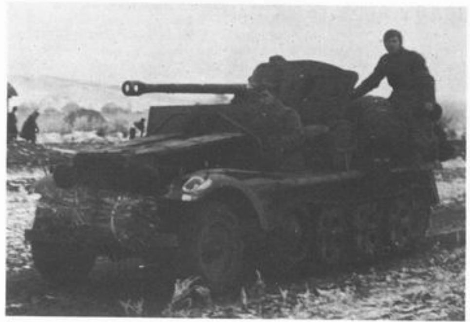
5cm Pak 38 (Sf) auf leichter Selbstfahrlafette To increase the mobility of the 5cm Pak, some of them were carried on the SdKfz 10 semi-tractor on a pedestal mounting. (Bundesarchiv, Koblenz)
