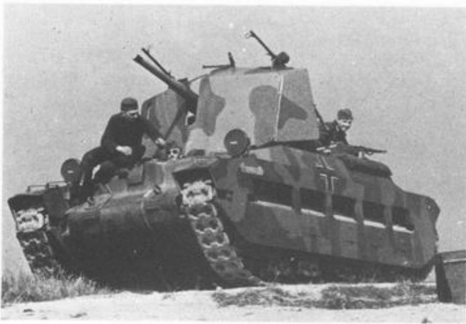
47cm Pak(f) auf Infanterie Panzerkampfwagen Mk II(e) Improvisation of the British Infantry Tank Mk II (Matilda) to mount the French 4,7mm anti-tank gun. Only one converted. (Bundesarchiv, Koblenz)
