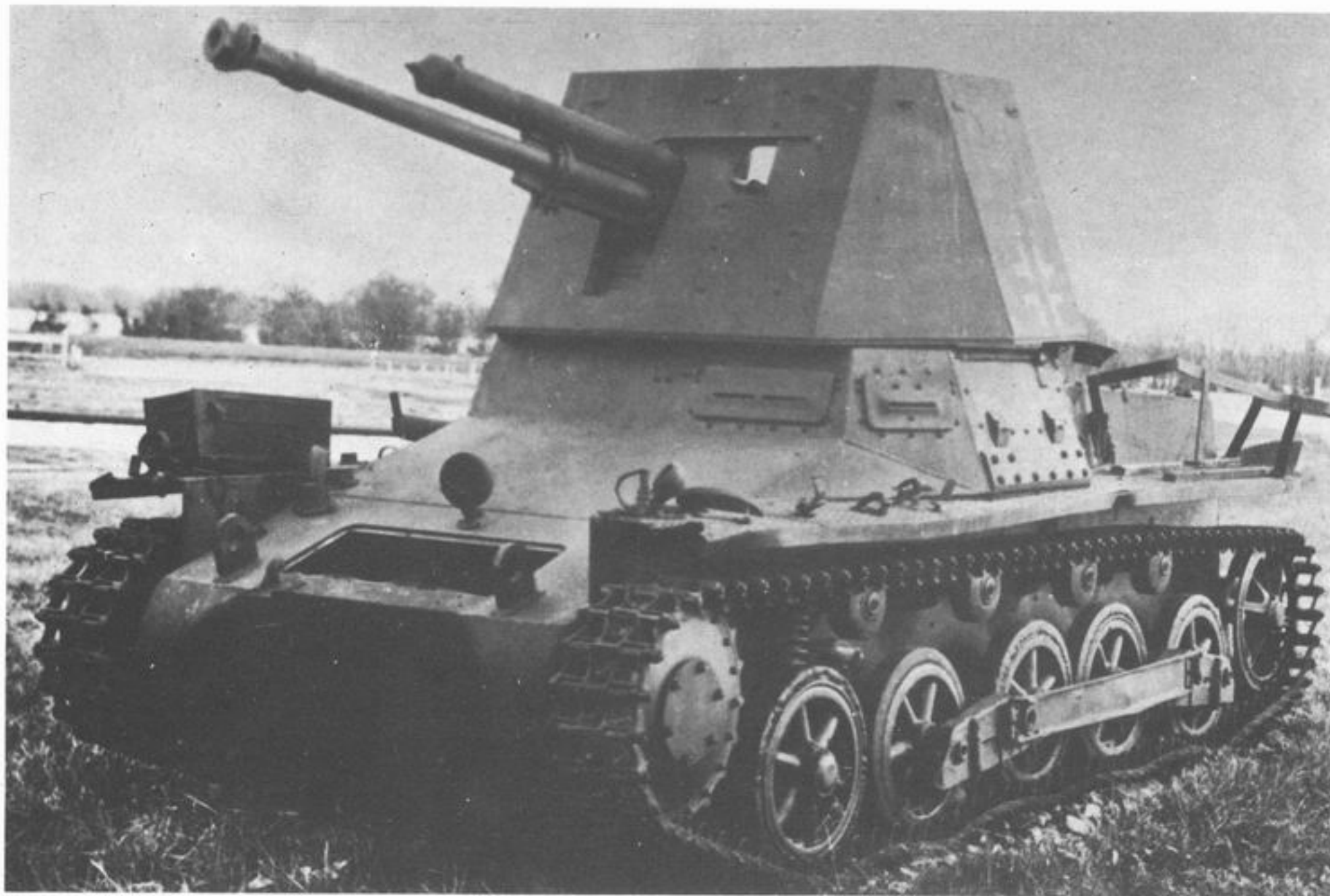
4,7cm Pak (t) Sfl auf PzKpfw I Ausf. B or Panzerjaeger I fuer 4,7cm Pak (t) Introduced into service in 1940, this was the first self-propelled anti-tank gun to enter German service. Based on the chassis of the Panzerkampfwagen I Ausf. B, this equipment was fitted with a Czech 4,7cm anti-tank gun L/43 mounted within a three-sided gun shield. Crew 3. Weight 6 tons.
