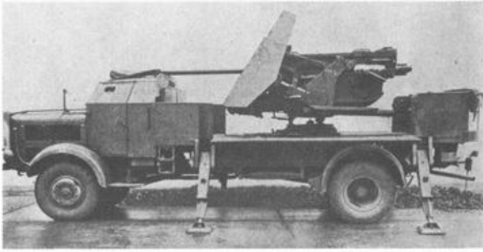
3,7cm Flak 36 auf Lkw Mercedes-Benz, 4500A 3,7cm Flak mounted on the chassis of the 4 × 4 Mercedes-Benz 4.5-ton cargo truck, Type 4500A. The vehicle was considerably modified for this adaptation.
