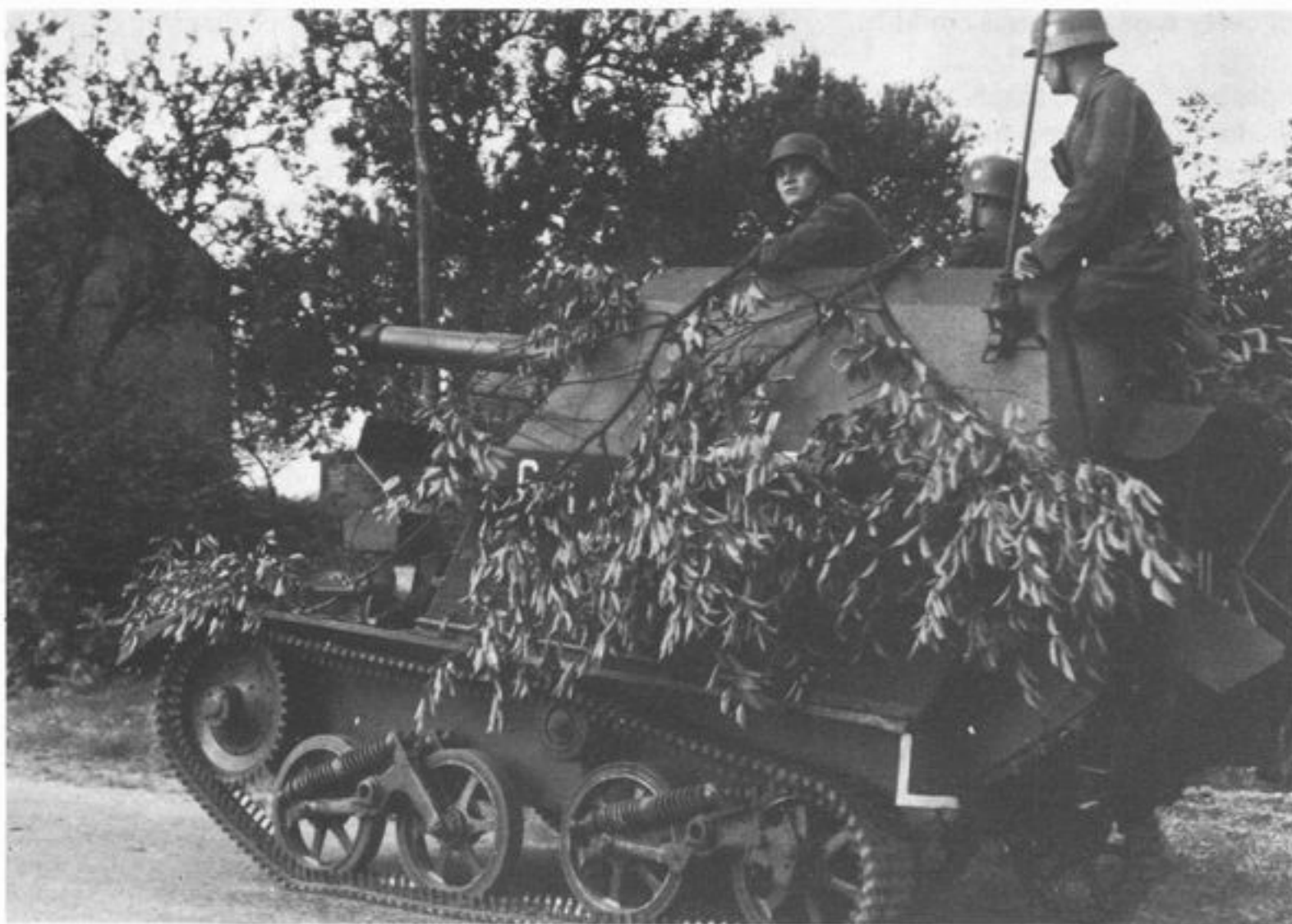
10.5cm (f) auf PzKpfw Mk VI (e) A small number of captured British light tanks of the Mk VI series were converted as mobile mounts for the French 105mm gun. (Bundesarchiv Koblenz)
