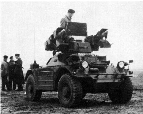
Ferret Mark 2 with Vigilant anti-tank guided missiles.
