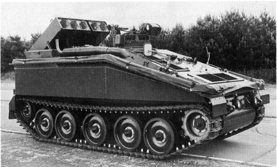
Prototype of Striker guided weapon vehicle with its five-Swingfire container elevated for firing.
