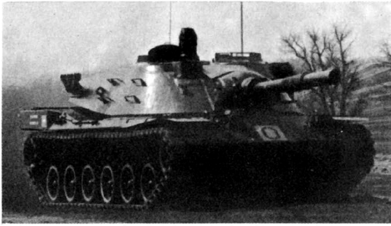
U.S. XM803, the "austere" version of the MBT-70 battle tank. (U.S. Army)
