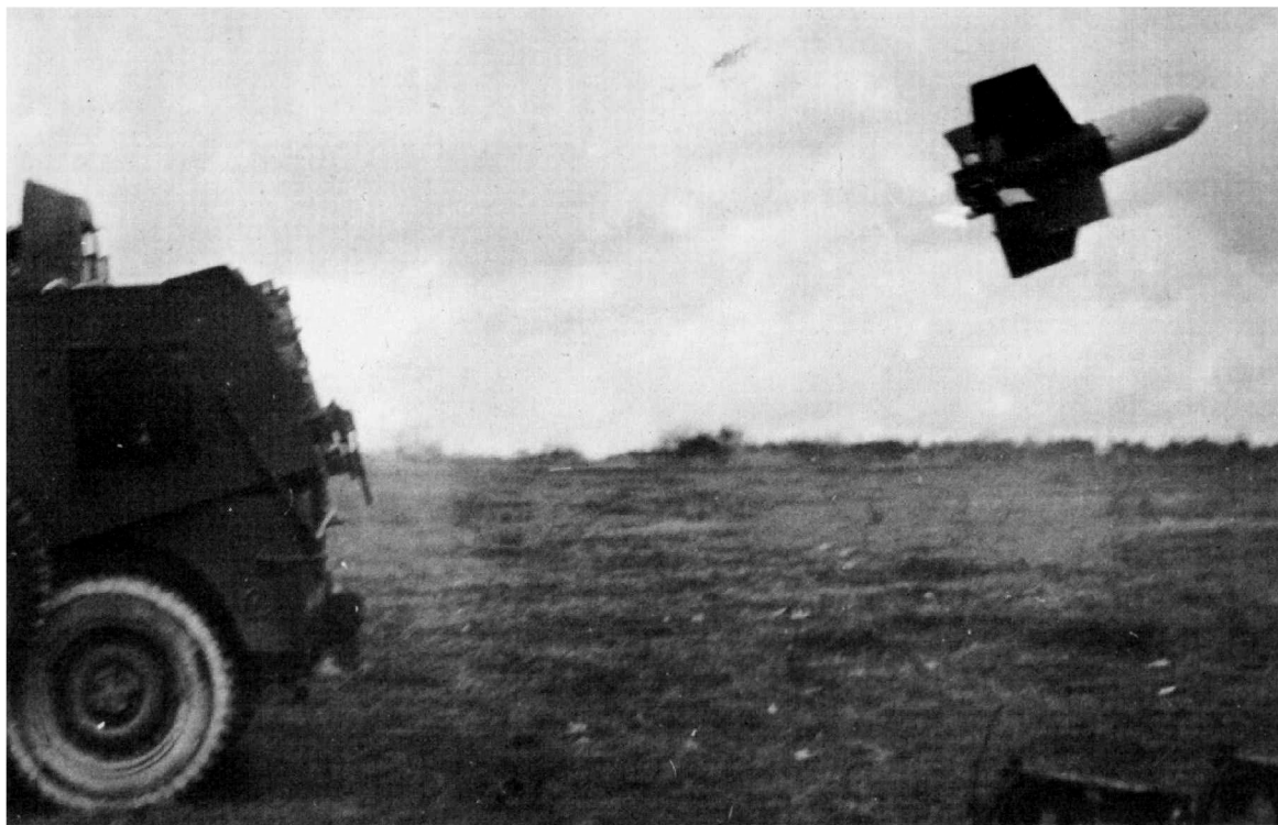
Nord-Aviation SS-10, the first anti-tank guided missile to go into service, fired from a jeep.
