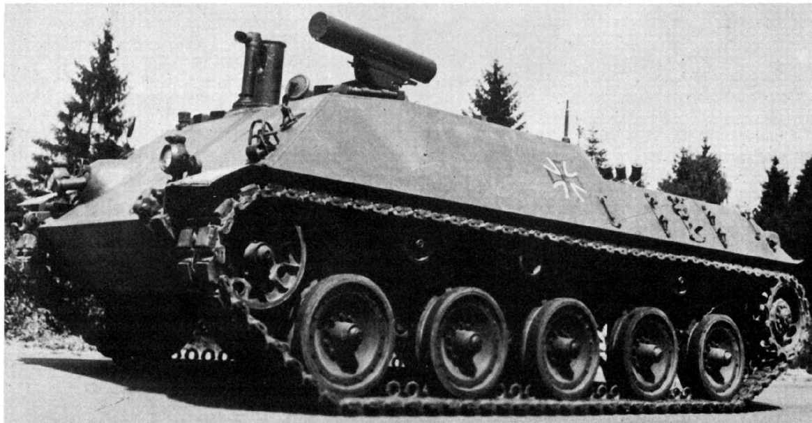
Second model of the Jagdpanzer Rakete with a HOT missile elevated into its firing position.
