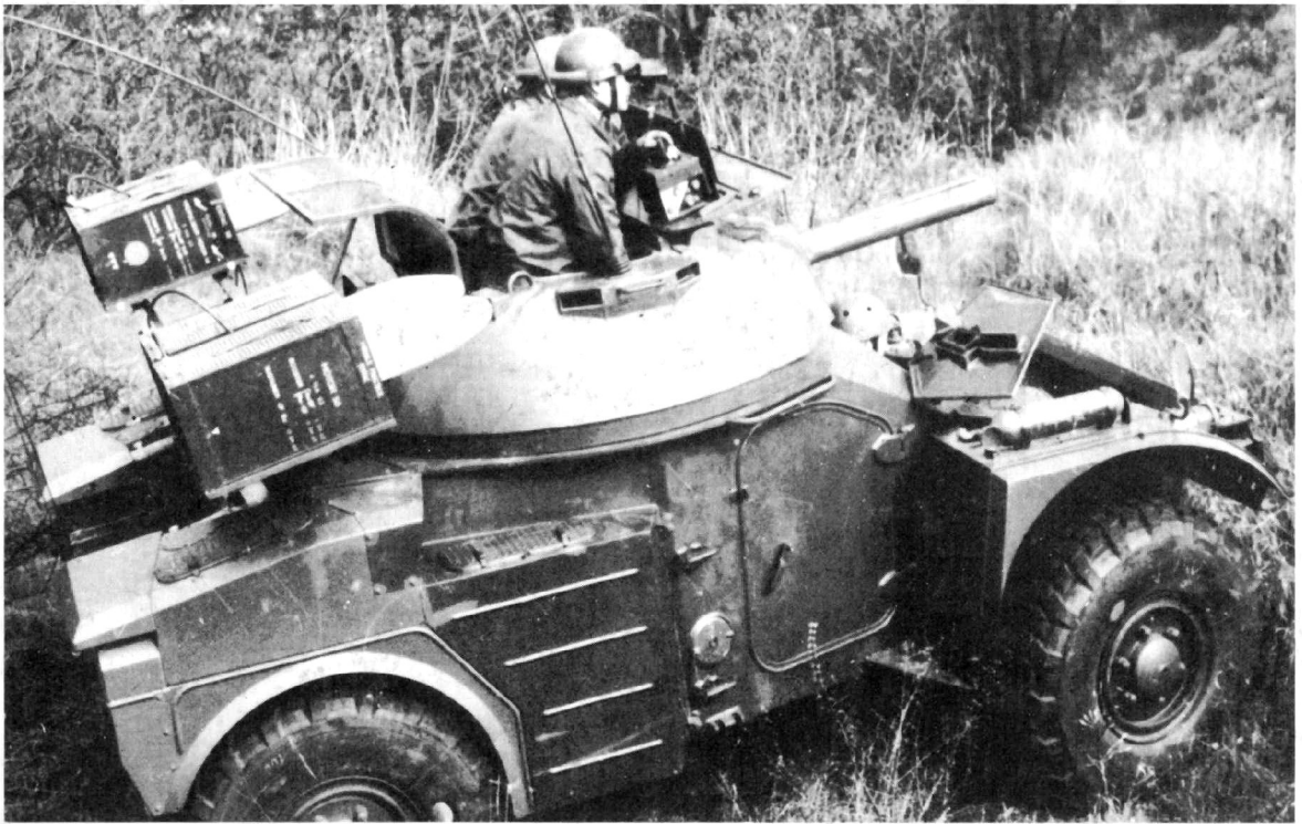
A.M.L. with HE.60 turret and S.A.M.O. 1160 launcher with ENTAC anti-tank guided missiles.
