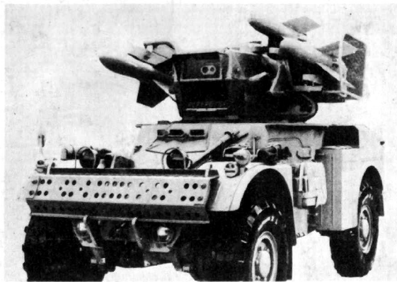
A.M.L. with H.90 turret and SS-11 missiles one of which has just been launched.
