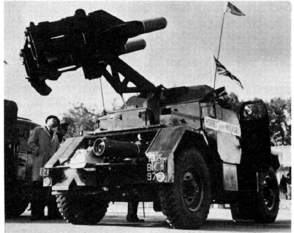
Hornet launcher vehicle with two Malkaras on its launcher arm and one stowed below it.
