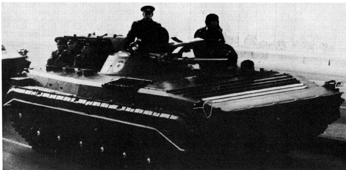
Soviet BMP-76 infantry combat vehicle with a Sagger missile above its 76 mm gun.
