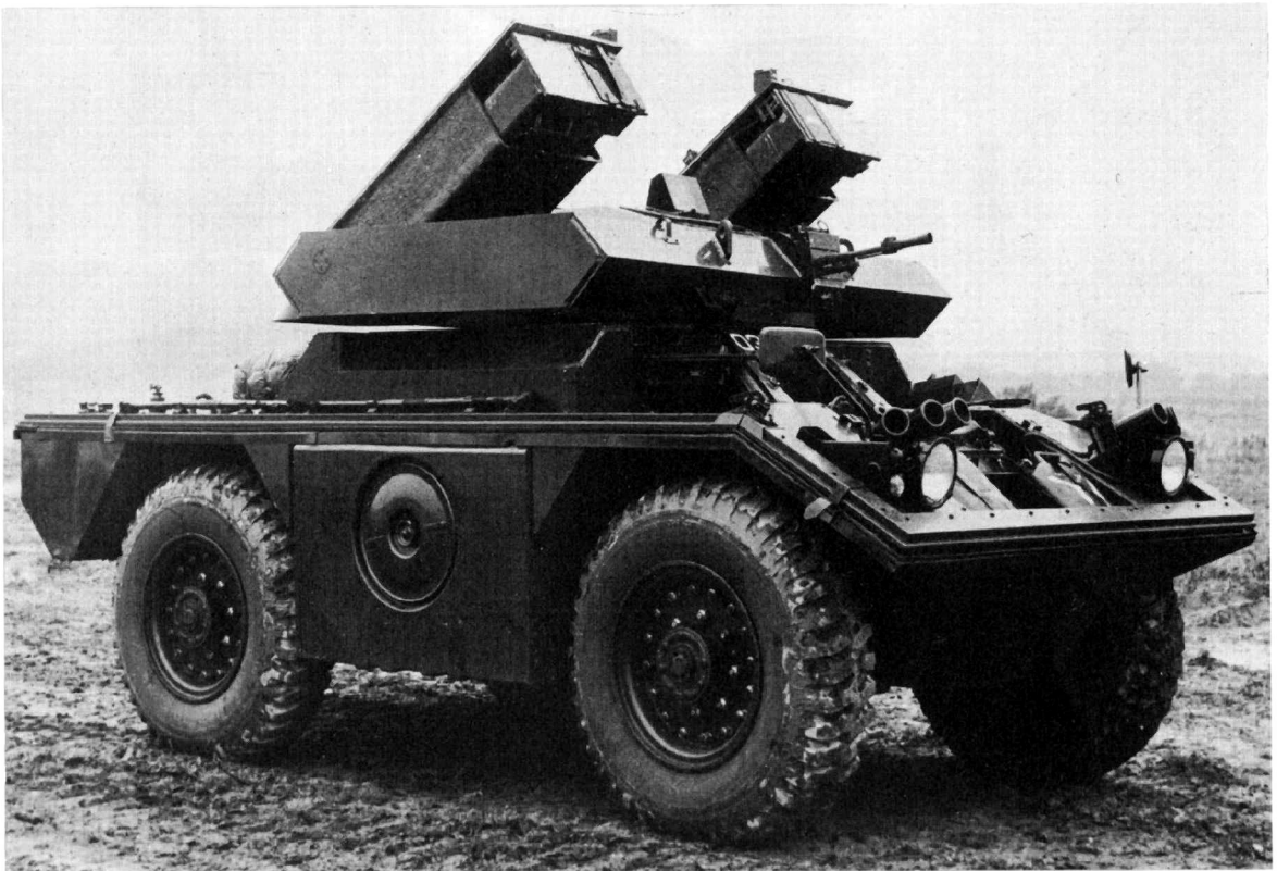
Prototype of Ferret Mark 5 with all four of its launcher boxes elevated for firing.
