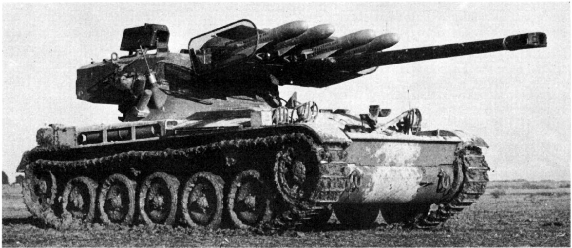
Harpon system consisting of SS-11 missiles with automatic guidance on an AMX-13: the missile tracker can be seen on top of the turret.
