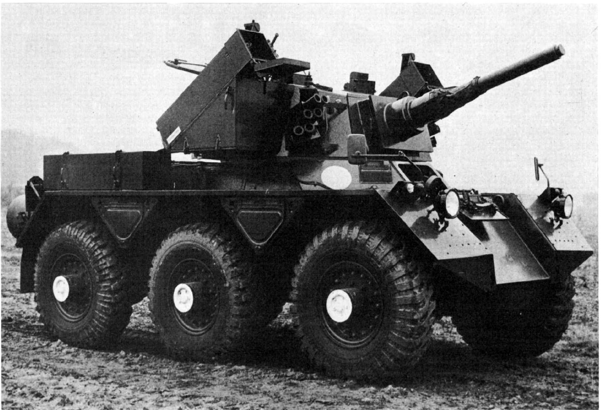
Saladin Mark 2 with Swingfire; two missiles are "ready-to-fire" on the sides of the turret, two are in containers on the rear wheelguards. (Alvis)
