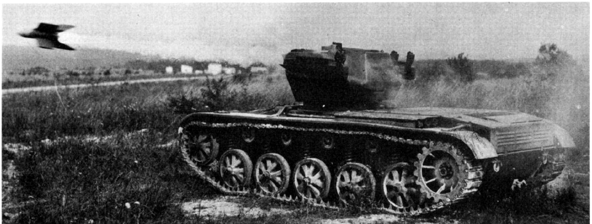
SS-11 fired from a NA-2 turret mounted on an Engin Léger de Combat . (Aérospatiale) (Note: A photograph of the NA-2 turret with one SS-12 and two SS-11 missiles on a Panhard AML appears in the Profile on Panhard Armoured Cars.)
