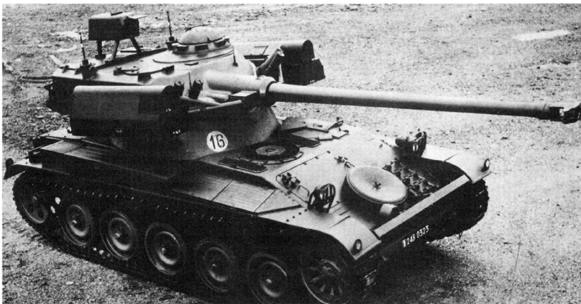
Triple HOT launchers on an AMX-13.
