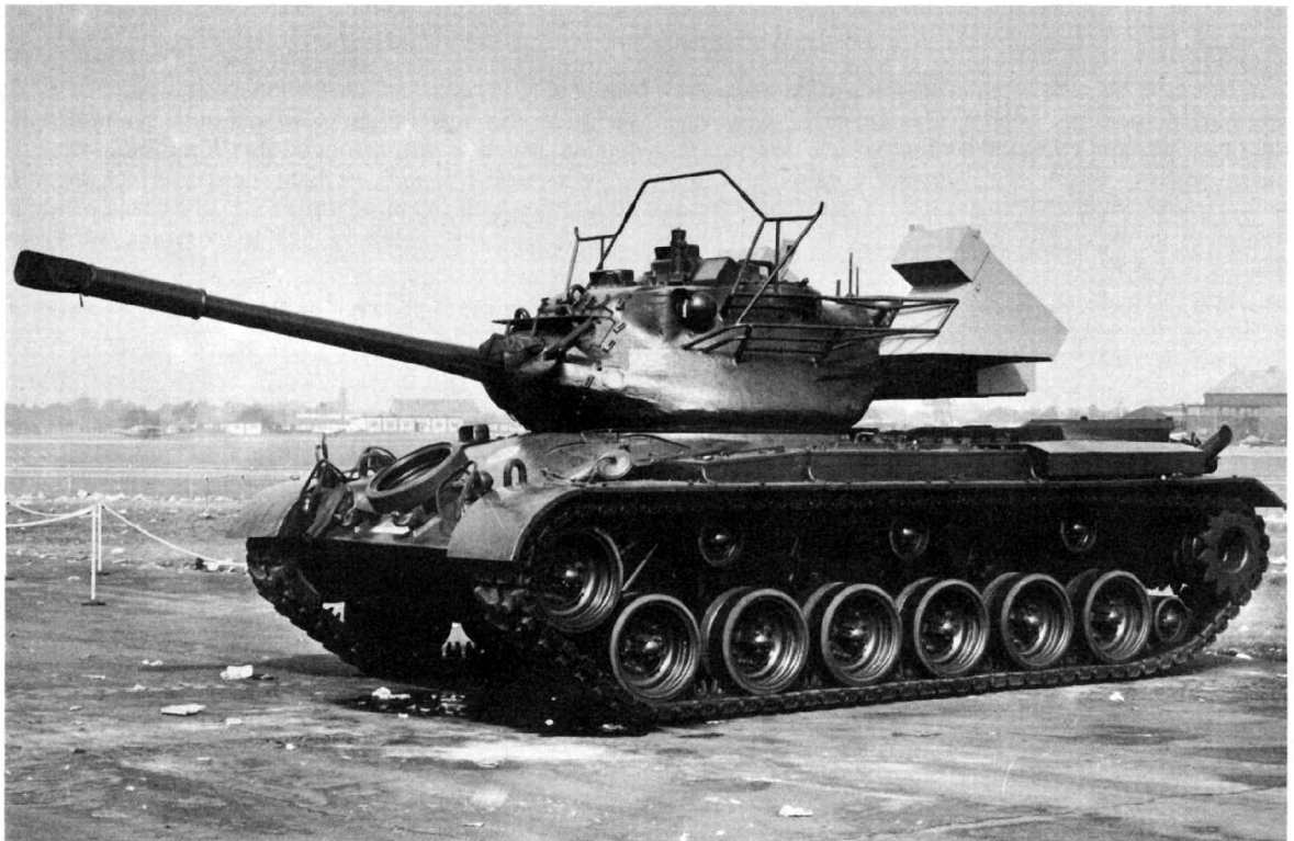
Mock-up Swingfire installation on an M47 medium tank.
