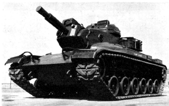
M60A1E2 battle tank with 152 mm gun/launcher. (Chrysler Corpn.)
