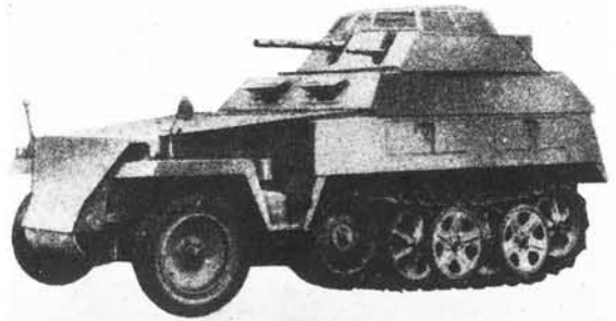
Late pattern SdKfz 250/9 with the new six-sided turret that was also being produced for the SdKfz 234/1 eight-wheeled armoured car. The vehicle also had the new pattern SdKfz 250 body.
