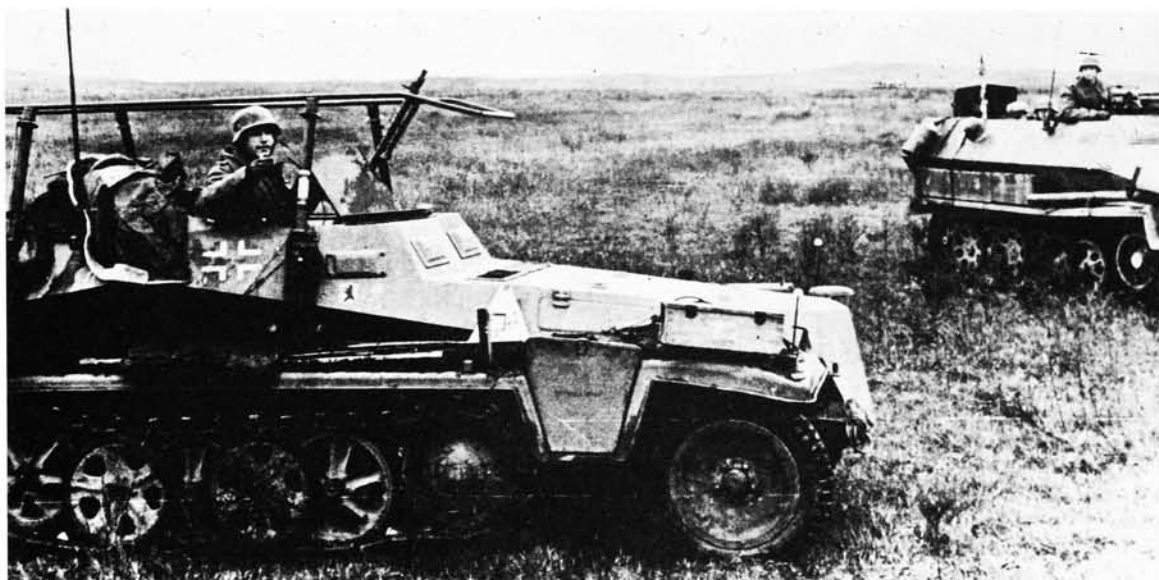
Leichter Funkpanzer SdKfz 250/3.III. This was one of the four radio vehicles that were among the variants of the Leichter Schützenpanzerwagen SdKfz 250. It carried a Fu 7 and a Fu 8, which was characterised by the frame antenna. It was used for ground-to-air communication.
