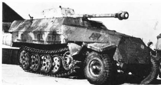
The version of the medium SPW SdKfz 251/22 mounted the 7.5 cm. Pak 40. This vehicle protected infantry against enemy tanks and appeared in ever-increasing numbers on the battlefield in 1944. (Col. Robert Icks)
