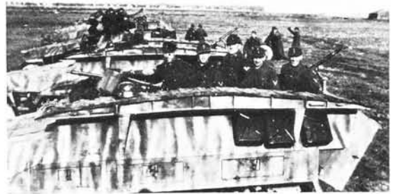
Engineer m.SPW Ausf. D, mounting bridging equipment and spare gasoline containers. They were used in numbers to assure mobility for tank formations. Mounting of both machine-gun 42s is clearly visible. (Col. Robert Icks)
