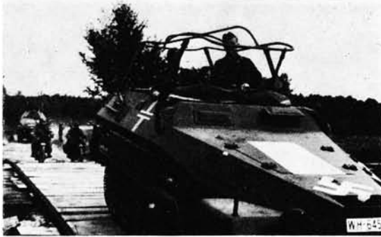
This unit, SdKfz 251/10, is equipped with the 3.7 cm. anti-tank gun and was issued to platoon leaders in 1940. It acted as a support vehicle until the 7.5 cm. gun became standard equipment. The chassis is that of an Ausf. A. (H. Nowarra)
