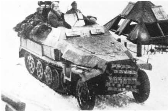
Engineer m.SPW Ausf. D, mounting bridging equipment and spare gasoline containers. They were used in numbers to assure mobility for tank formations. Mounting of both machine-gun 42s is clearly visible. (Col. Robert Icks)
