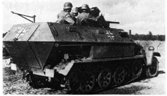
This unit, SdKfz 251/10, is equipped with the 3.7 cm. anti-tank gun and was issued to platoon leaders in 1940. It acted as a support vehicle until the 7.5 cm. gun became standard equipment. The chassis is that of an Ausf. A. (H. Nowarra)
