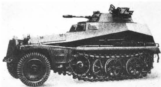
SdKfz 250/10 was armed with a 3.7 cm. Pak instead of the forward MG. (below)
