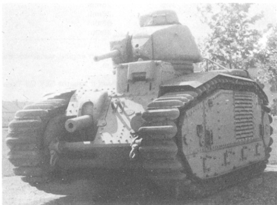
2 This Char B1 bis, captured from the Germans and now in the RAC Tank Museum, Bovington, Dorset, bears the letter abbreviation for 'School of Tank Technology'. Note the slits for periscopic binoculars in the cupola, revealed by the raised visor. (RAC Tank Museum)
