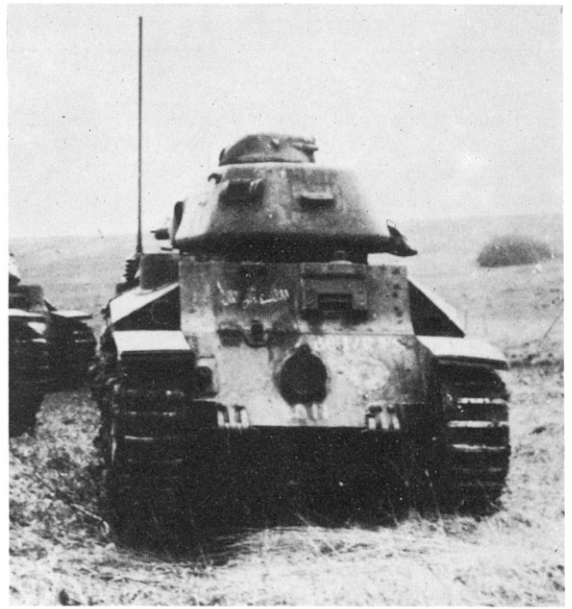
1 The Renault Char D2 was a 20-ton medium tank for the infantry which provided the basis for the design of the cavalry's S35, but in technical detail and construction the two tanks were very different. Although fairly well armoured (40 mm), the Char D2 offered an almost vertical front hull face. (E. C. Armées)
