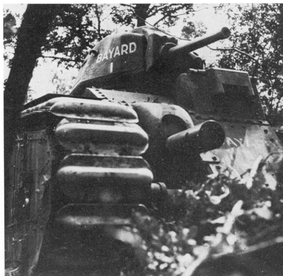
The heavily armoured Char B1 bis, with its 75mm gun in the hull and a turret-mounted anti-tank gun, was regarded at the outbreak of World War II as one of the most formidable tanks in service anywhere.
