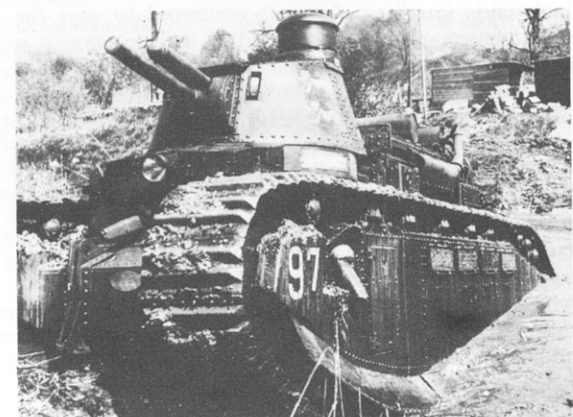
Char 2C climbing the bank of a stream. Note the brackets in centre front hull for slinging on to special rail wagons. This tank, named 'Normandie', has the arms of the Province painted on the turret.
