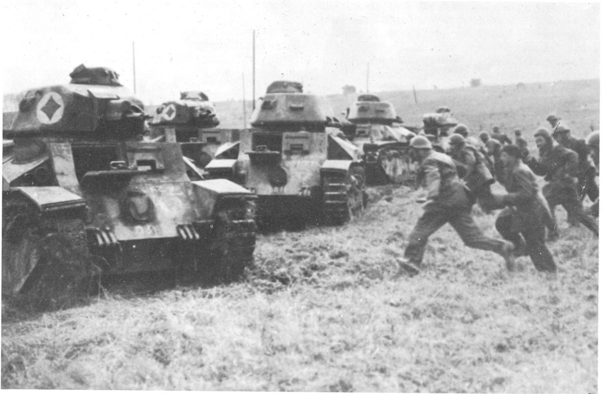
'Crews Mount! The main entrance to the Char D2 was in front of the wireless operator's position.
