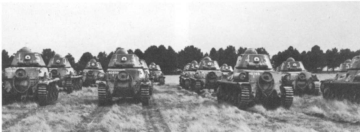
H 35s, clearly showing the downward slope of the engine deck—a main recognition point between the H 35 and the H 39. (E. C. Armées)
