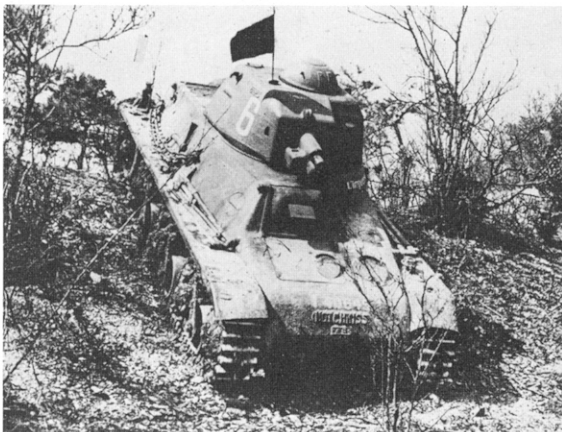
An H 39, in comparison with the R 35, indicating a recognition point with the driver sitting on the right side of the tank.
