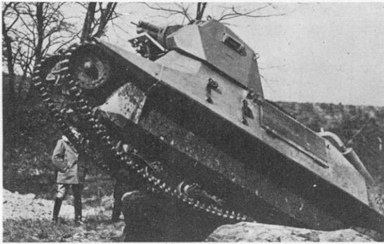
The F.C.M. 36 was different in almost every respect from other French light tanks, although armed with the same 1918 model 37mm gun and machine-gun. (E. C. Armées)
