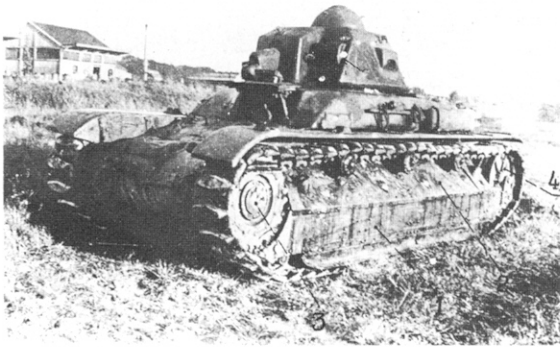
A prototype of the R 40, with lower skirting plates, three top rollers, spudded tracks, and a light shield covering the bogie wheels.
