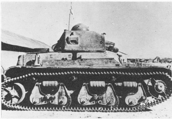
The suspension of the R 35, with bogies arranged in pairs or singly on bell cranks and with rubber springs, was similar to that of all the cavalry's auto-mitrailleuses.
