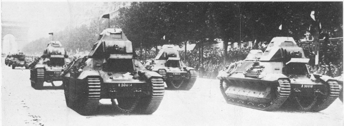
A diesel engine gave the F.C.M. 36 a reasonable speed and a good radius of action (225 kms.). These F.C.M. 36 tanks are in the 1939 Bastille Day parade. The Arc de Triomphe in the background. (I.W.M.)
