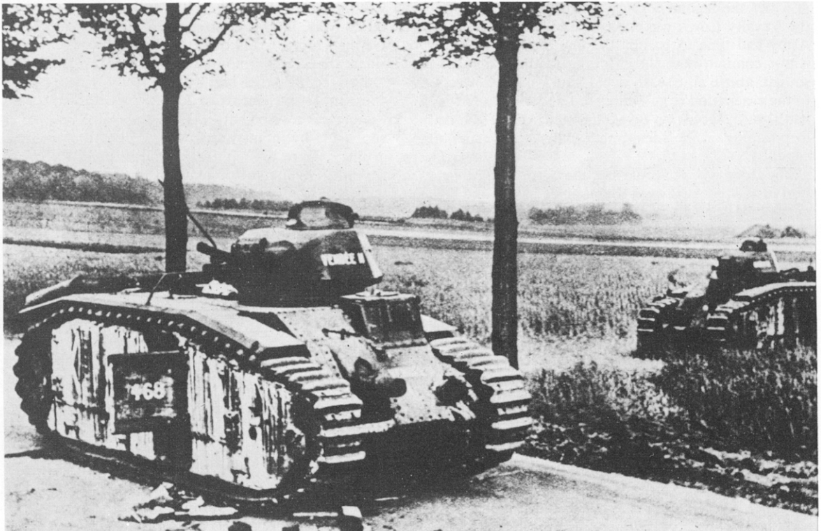
Knocked out and, perhaps, short of fuel. The Char B1 bis was not designed for the mobility of armoured warfare exemplified in the German Blitzkrieg.
