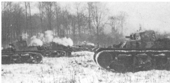
The suspension of the A.M.R. Renault 35 ZT was very similar to that adopted for the R 35, but with four wheels instead of five. (E. C. Armées)
