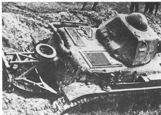
An R 35 apparently bogged down in the mud. Note the grills in the engine deck for air-flow through the radiator, and the stowage bins on the track guard (which were not carried on the Hotchkiss tanks).
