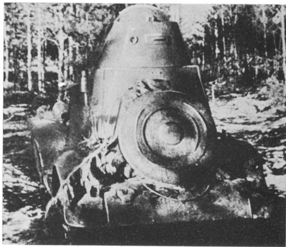
Rear view of BA-20M. This new model of the BA-20 was welded throughout—another point of recognition as well as its whip-type aerial on the left-hand side.
