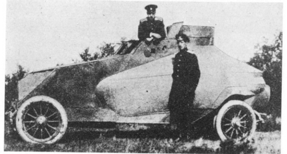
Austin armoured car with diagonally-arranged turrets, armoured in Russia at the Putilov works.
