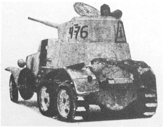
Three-quarter left rear view of BA-10 showing tracks fitted round its rear wheels for cross-country movement. All the six-wheeled armoured cars could be similarly fitted.
