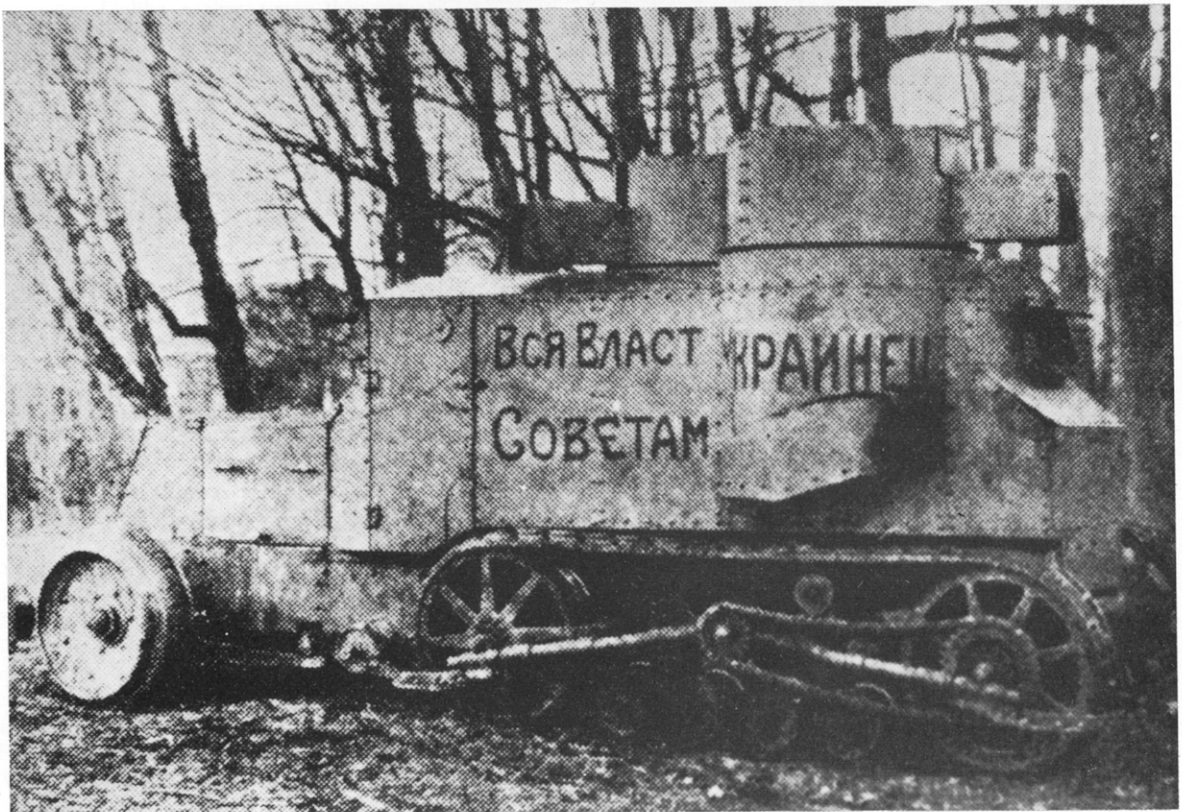
Austin-Putilov half-tracked armoured car. The small wheels in front were added to improve obstacle-crossing ability. This model had diagonally-arranged turrets.
