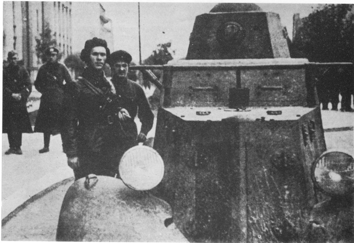
BA-20V with frame aerial round the hull. The BA-20 was a re-designed version of the Bronieford.
