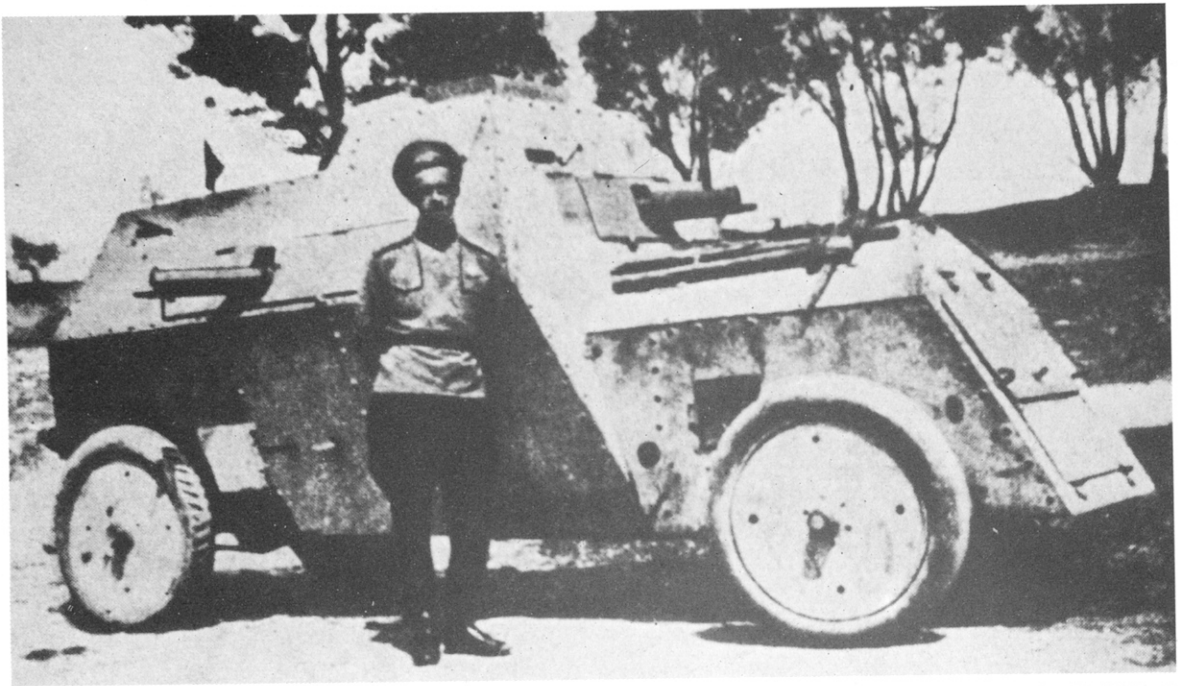
The Russo-Baltic armoured car had three machine-guns—one at each side and one in the front of a fixed turret. The first was built before World War I.
