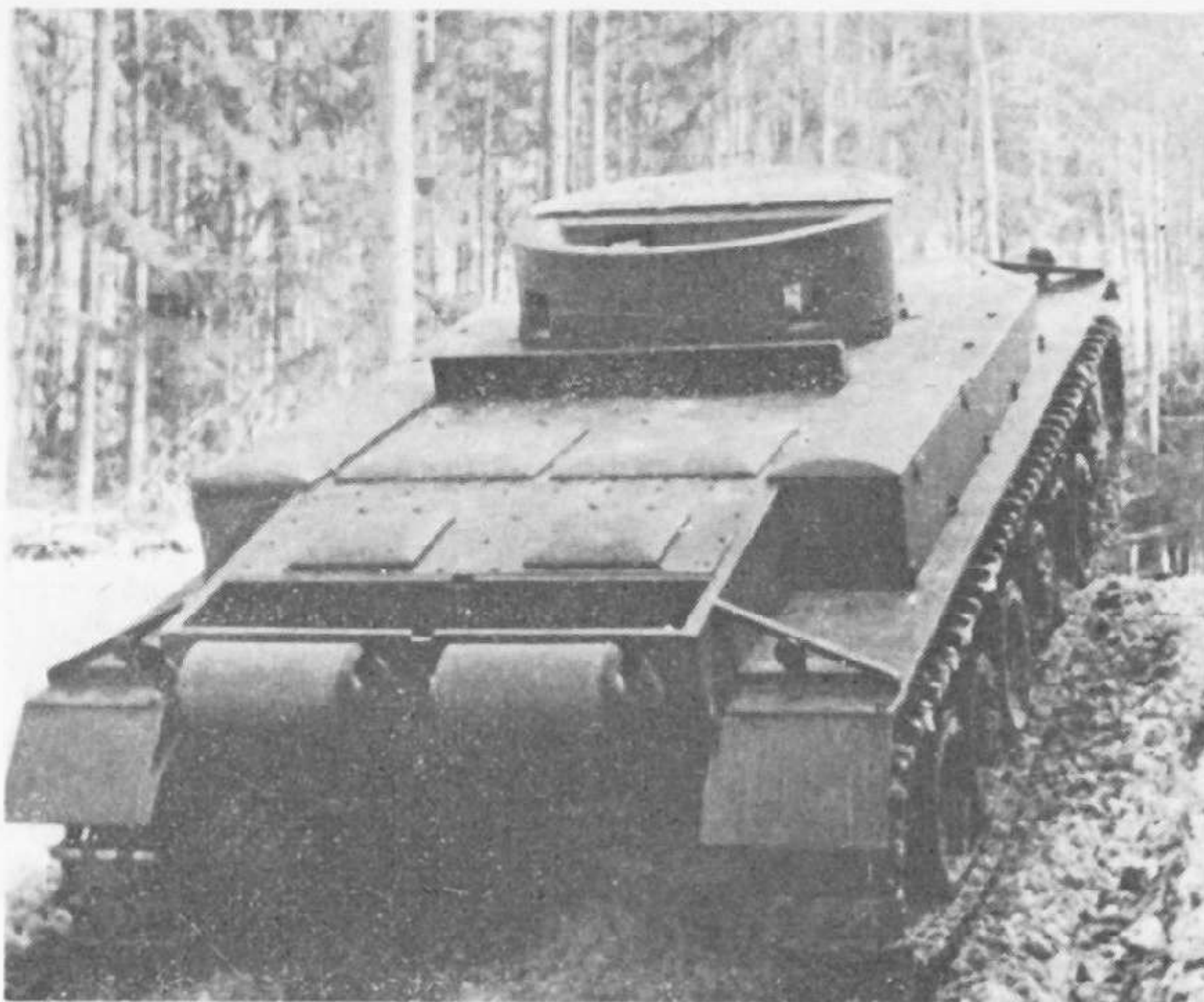
This unit was intended to replace the Panzer IV and was equipped with two air-cooled V-10 engines which drove electrically the two front sprockets.
