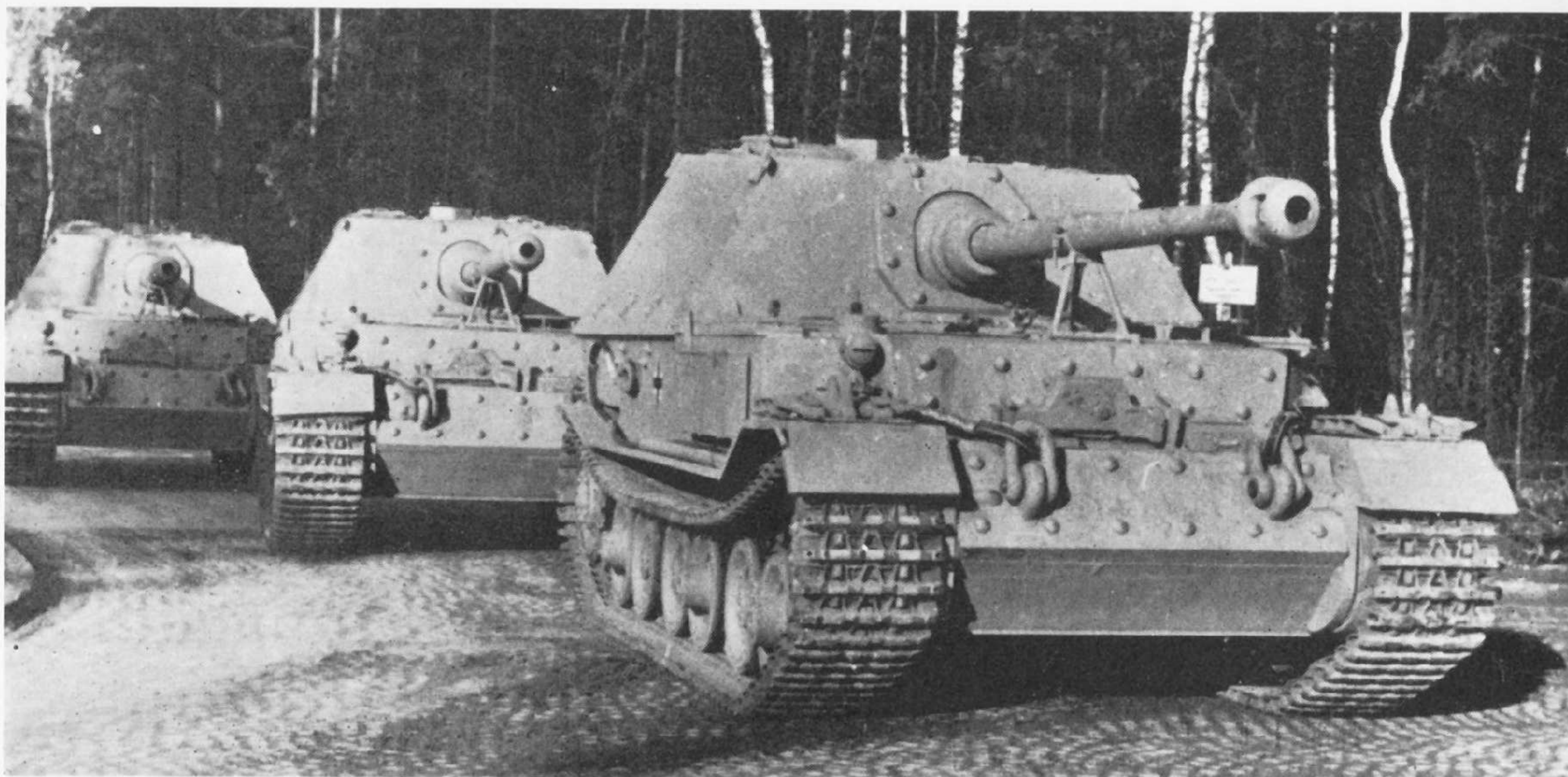
Three new Elefants of the first production run during test trials at the Alkett factory in Berlin. The gun mantlet is without the additional protection applied later on.
