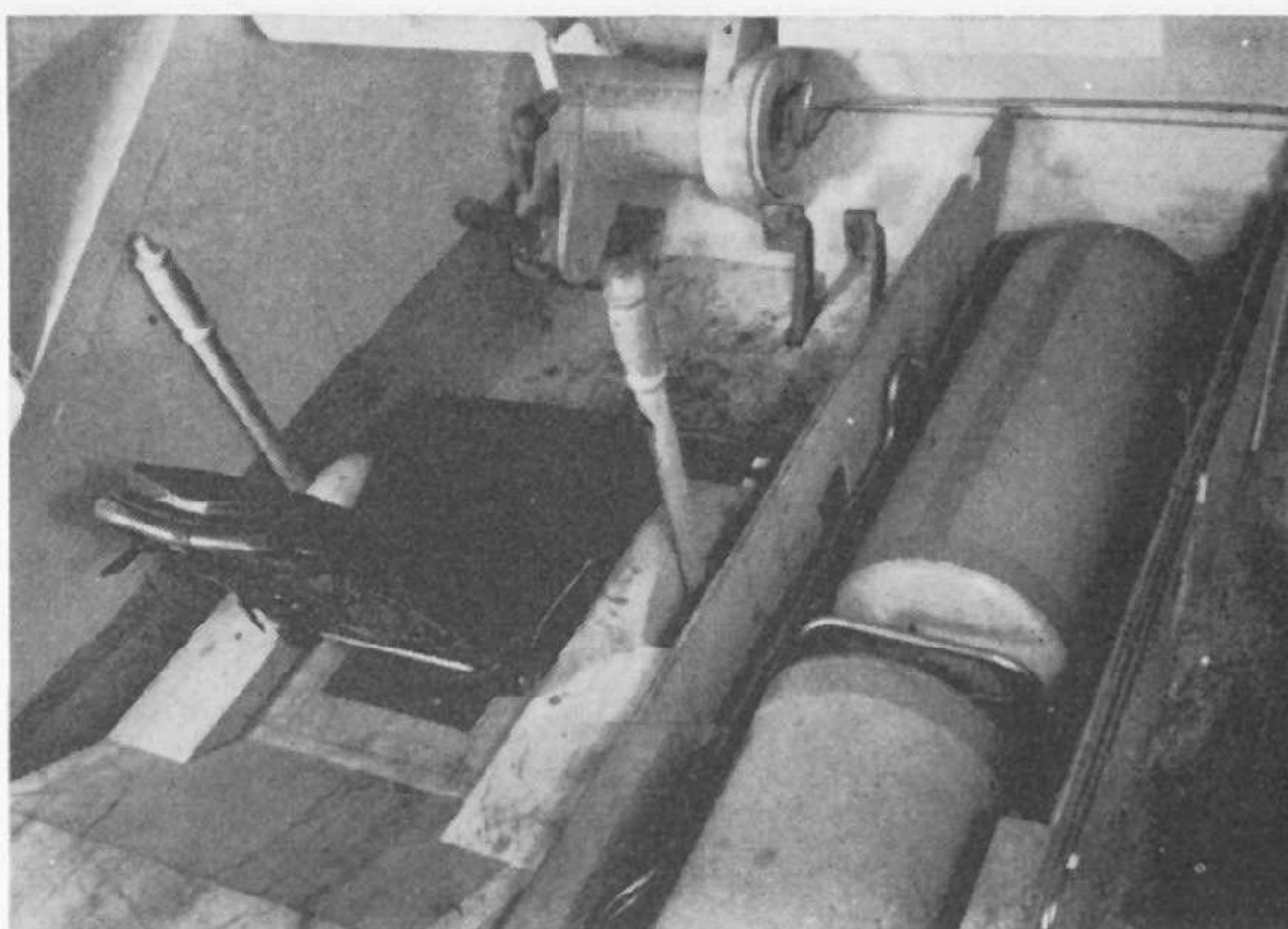
A wooden mock-up of the Porsche Tiger hull with a spacious driver compartment showing the air tanks for the hydro-pneumatic steering system.
