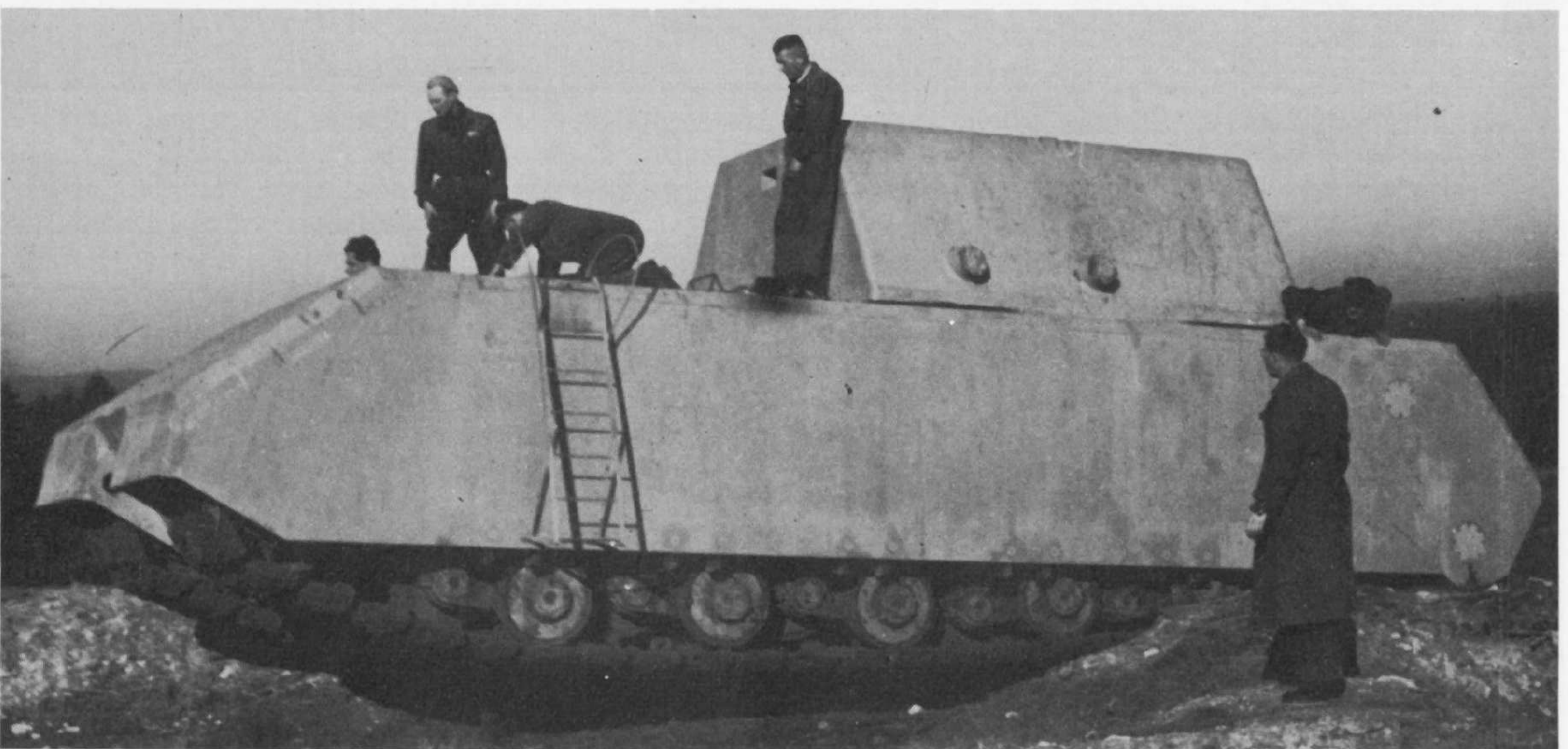
Five views of the Maus during its trials, with a 55-ton weight set on the superstructure towards the rear of the vehicle to simulate the turret which was not yet completed. It was over 30 ft. long.
