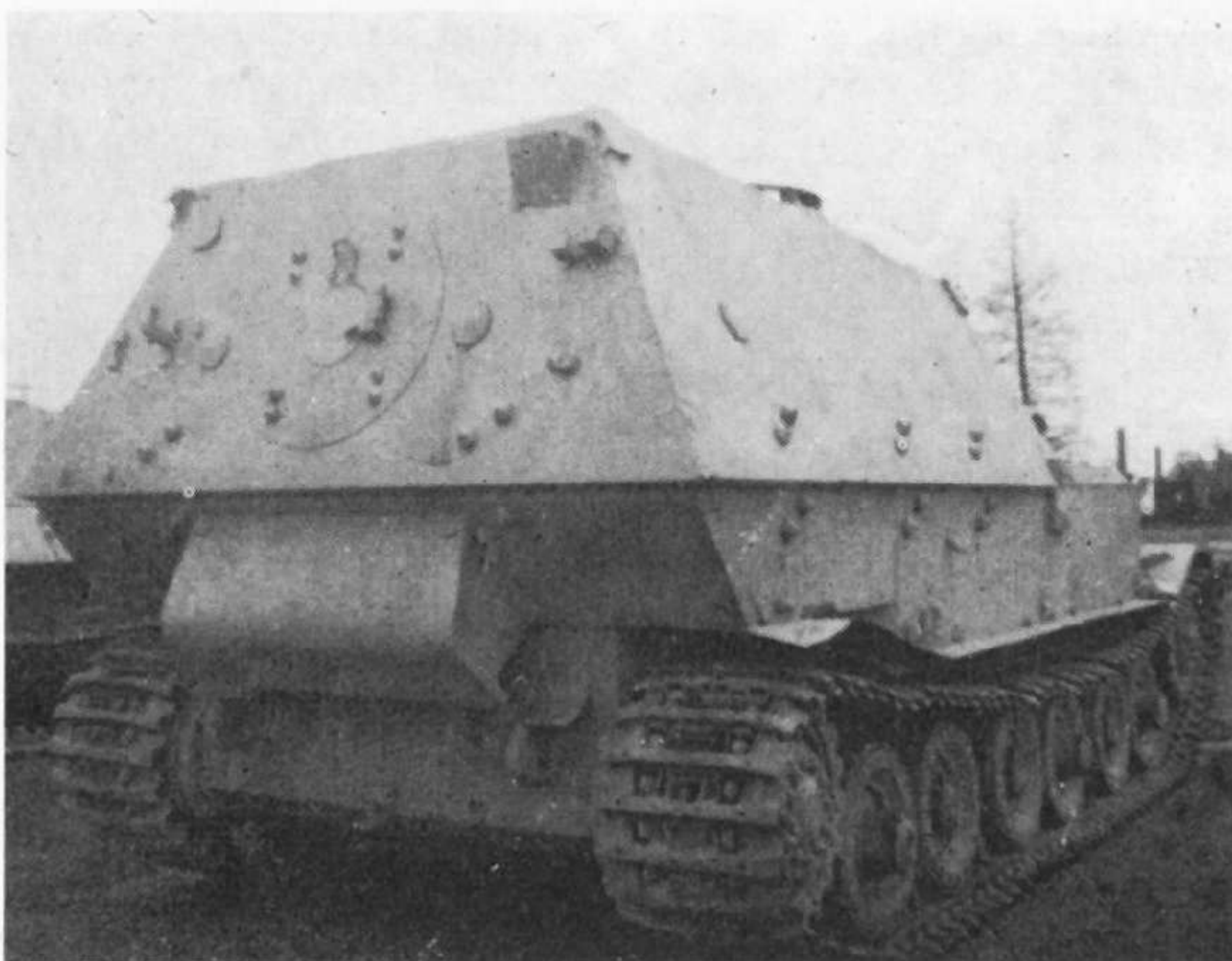
A rear view of the Elefant preserved at the Aberdeen Proving Grounds, shows the interlocking armour plates of the superstructure used on most German vehicles from 1943. The concentric hatches in the rear plate of the superstructure served for the ejection of empty cartridges during combat, and also (the larger one) for the removal of the gun.
