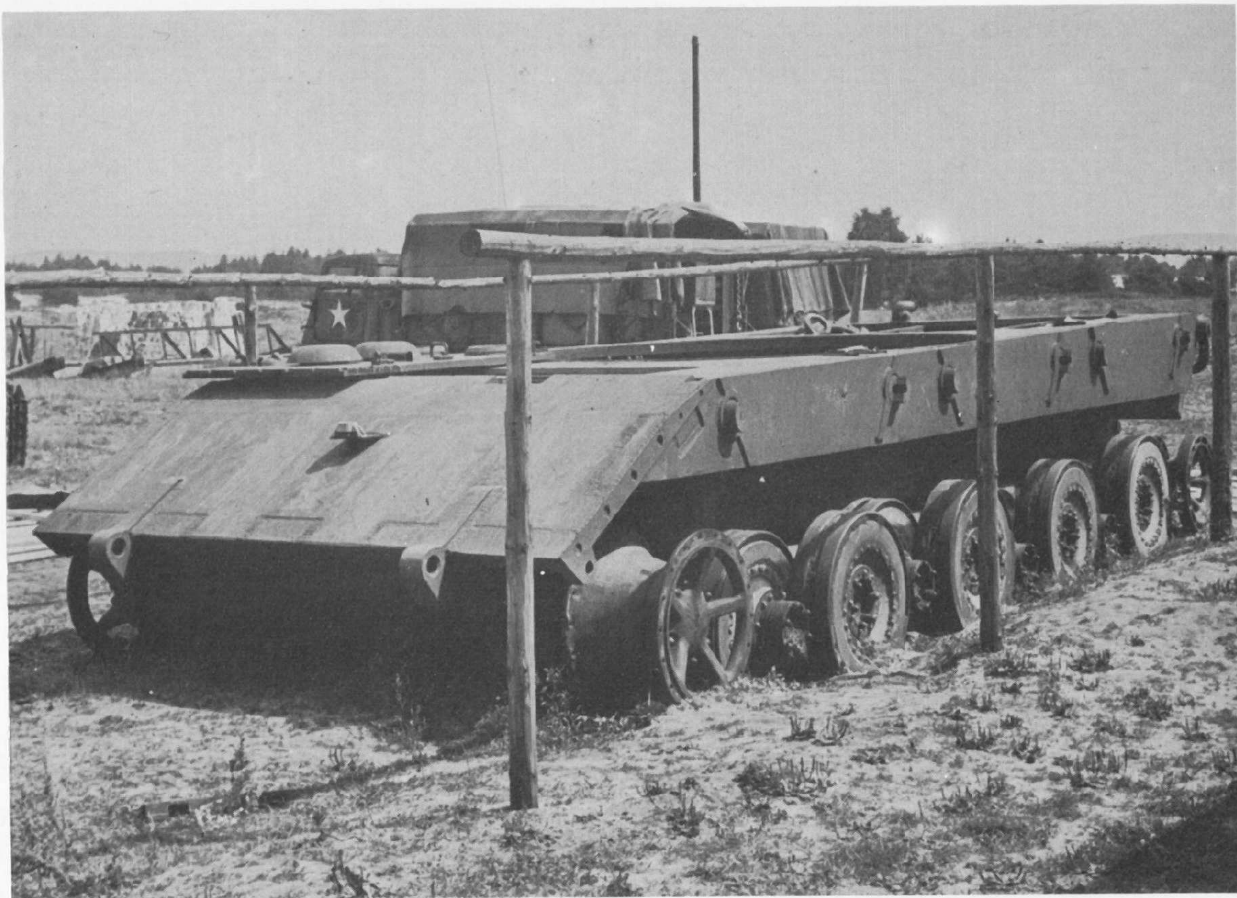
Assembly of the E-100 prototype was not complete when the war ended in May 1945. The partially finished vehicle was captured by the Allies. It was 869 cm long (without barrel overhang)
