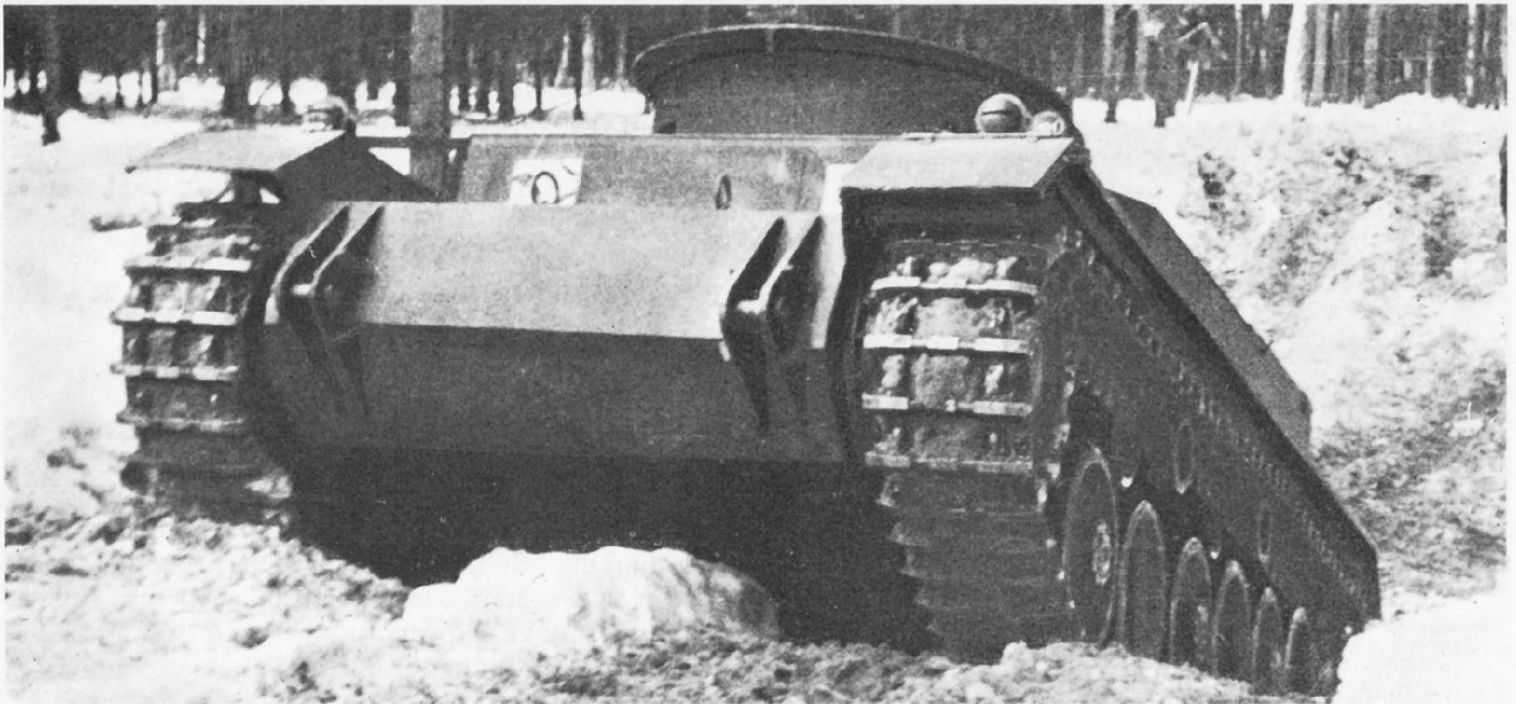
Professor Porsche's first attempt to create an armoured fighting vehicle resulted in two prototypes of the Porsche Type 100 or, as it was internally called, the "Leopard".
