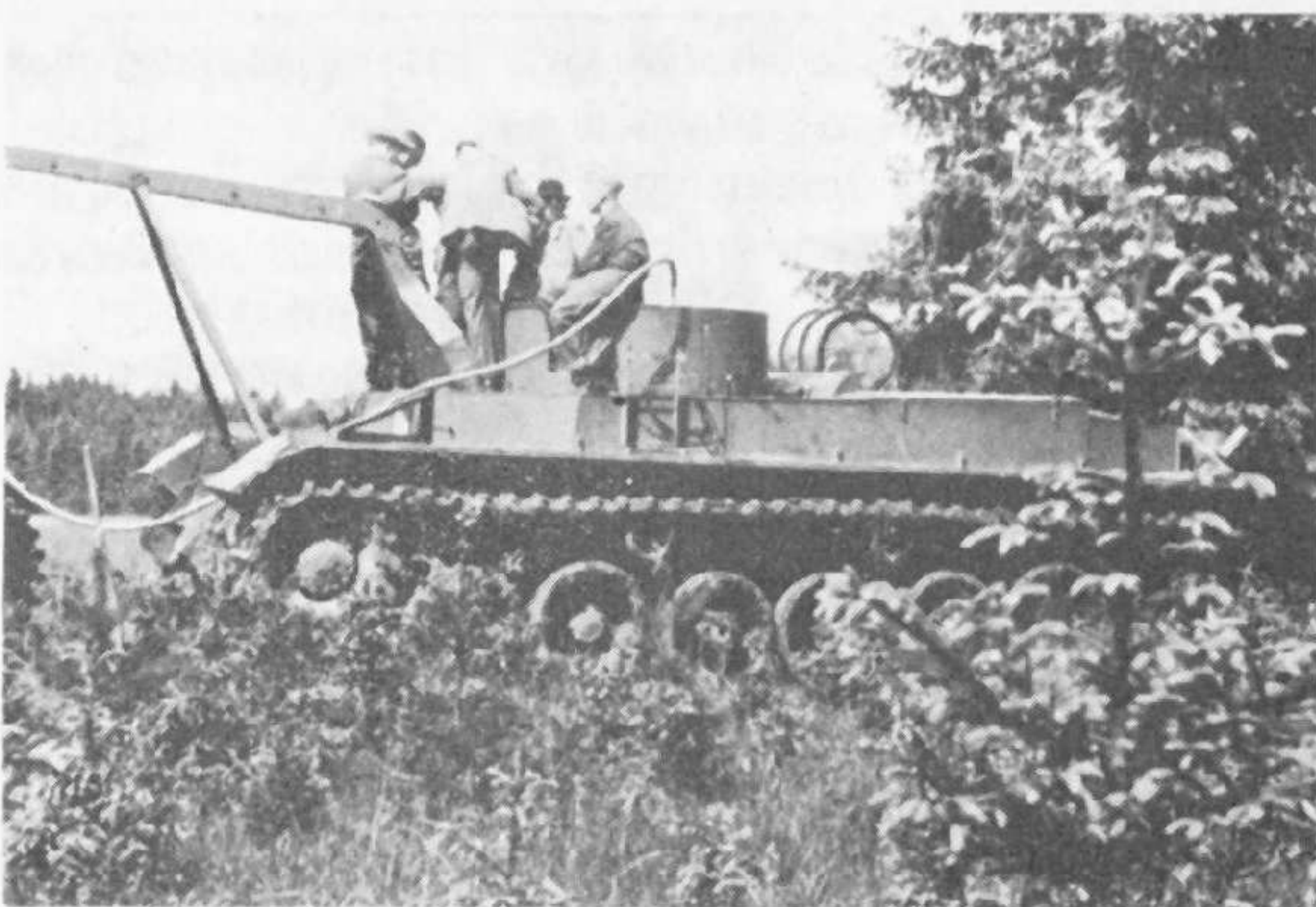
During intensive field trials the Porshe Type 100 was also used to supply the Porshe Type 101 with electric current during the initial field testing of the Porshe Tiger.
