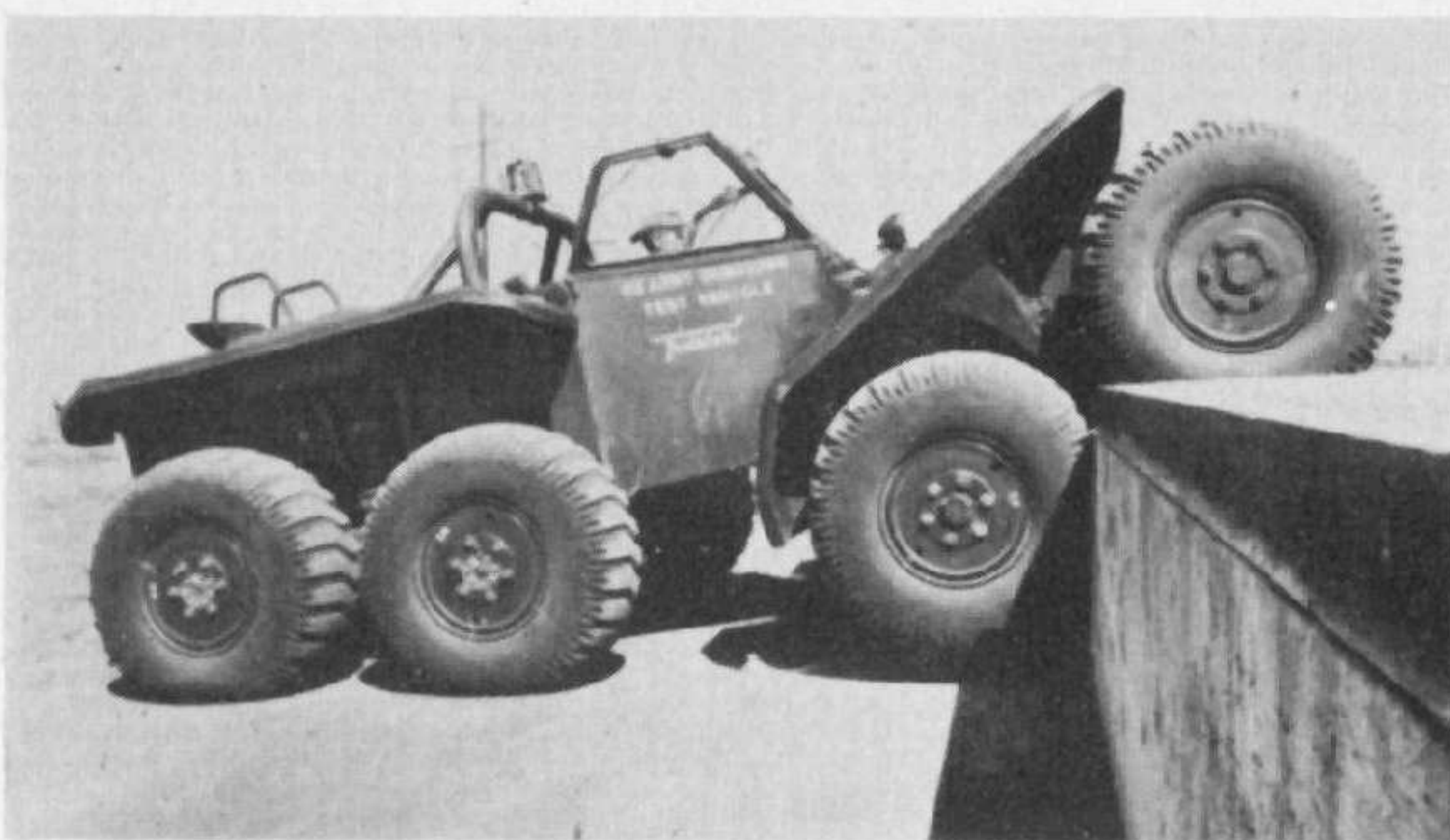
The U.S. Army's first Twister climbing a 3-foot vertical wall—October 1969.
