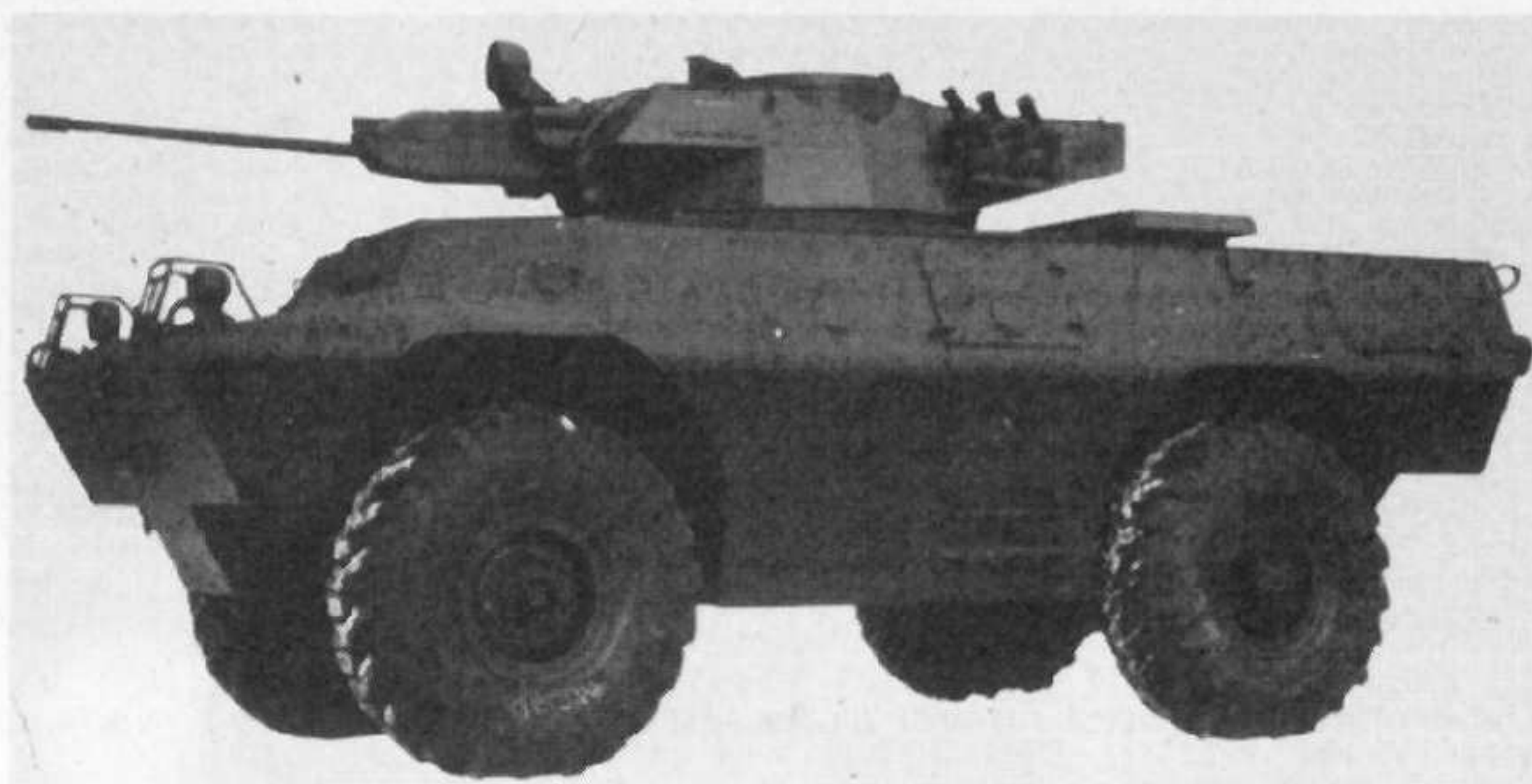
The V-200 Commando with a turret-mounted 20mm gun and six smoke dischargers each side of the turret rear.
