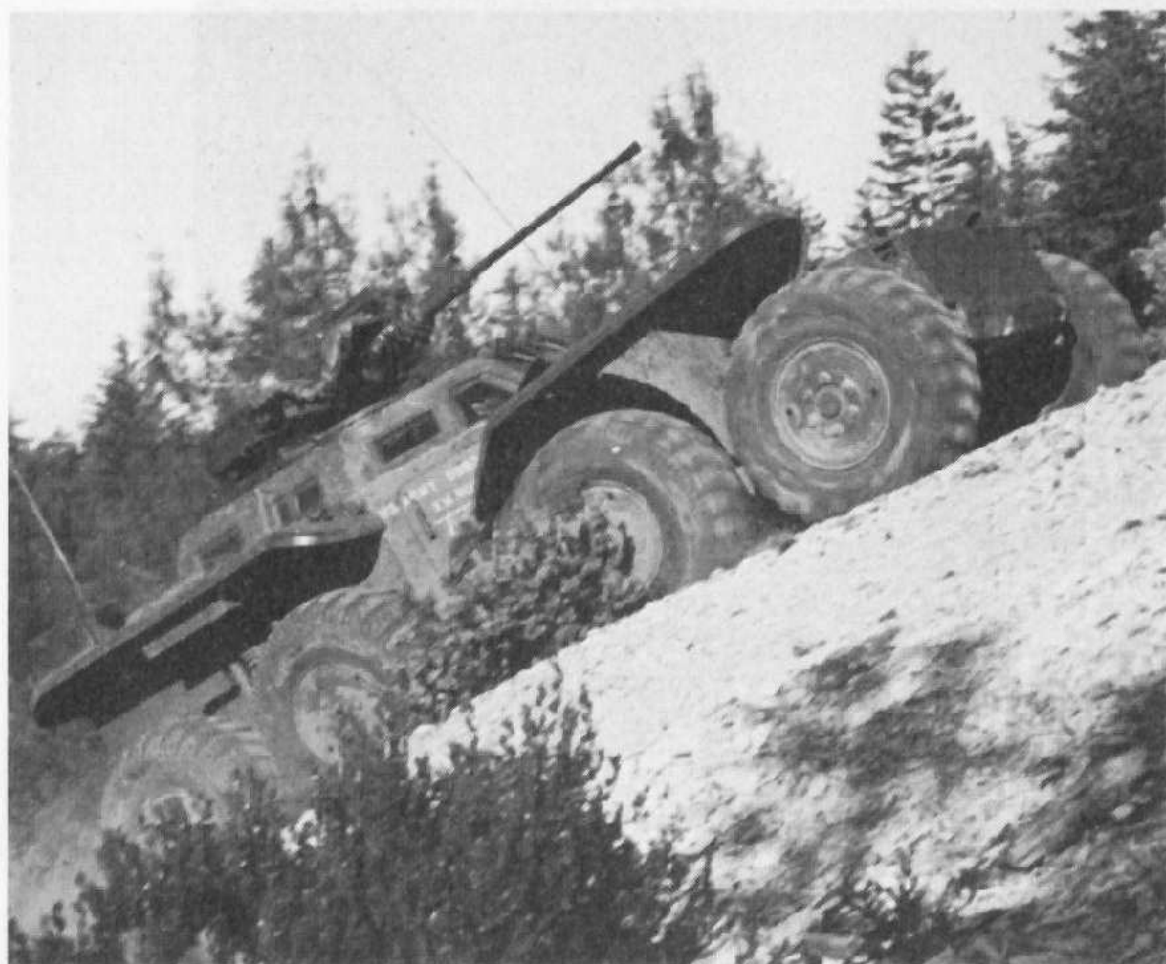
The armoured Twister, XM808, climbing a steep slope. Note the 20mm cannon. (Lockheed Missile & Space Co.)
