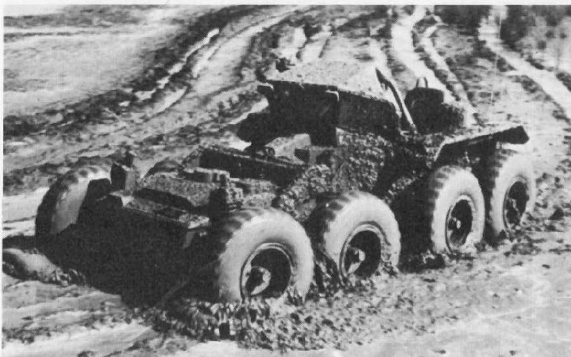
The original Twister showing its ability to move through mud.
