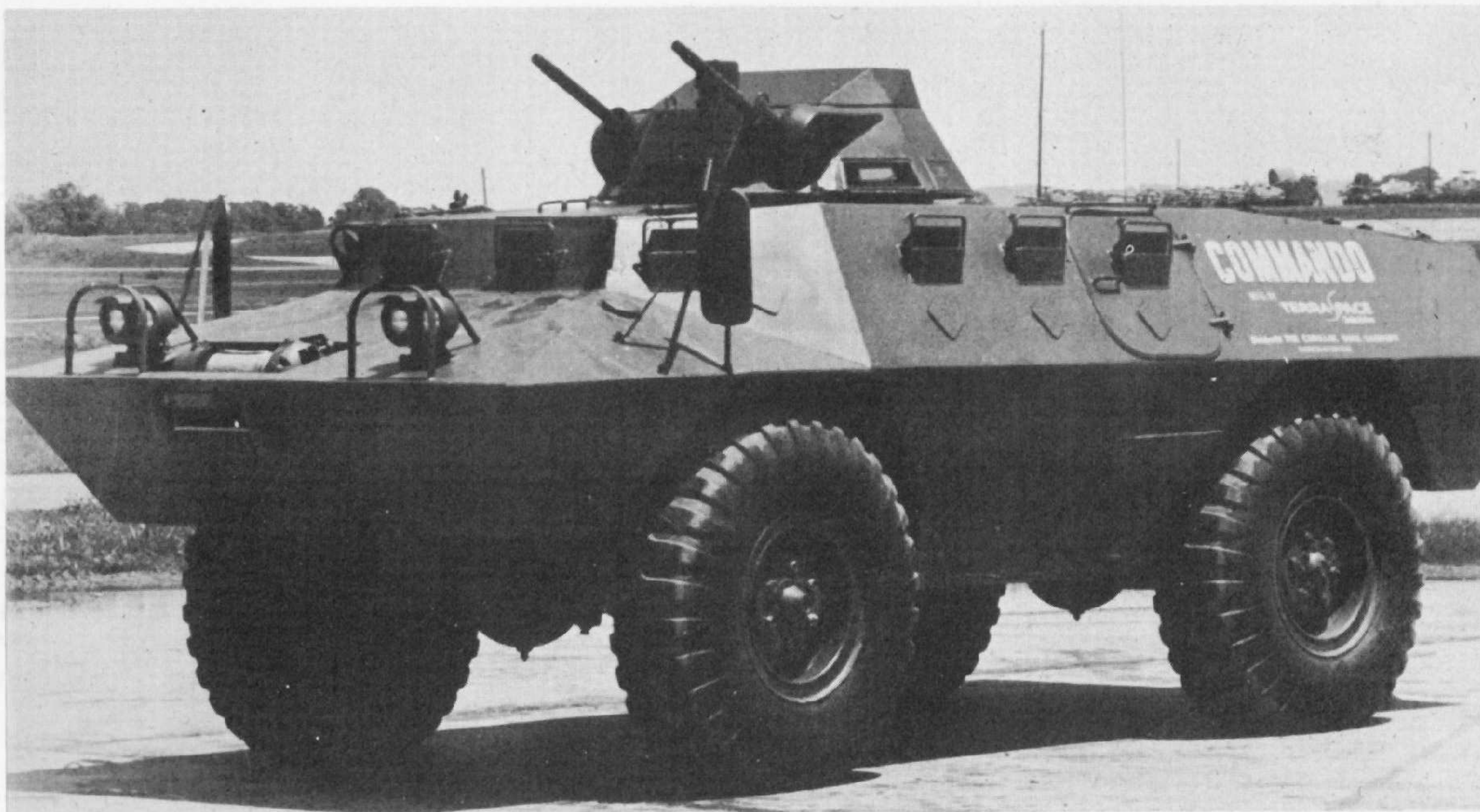
One of the early Commando vehicles (Car Armored Light 4x4 "Commando"). Note the different vision devices.
