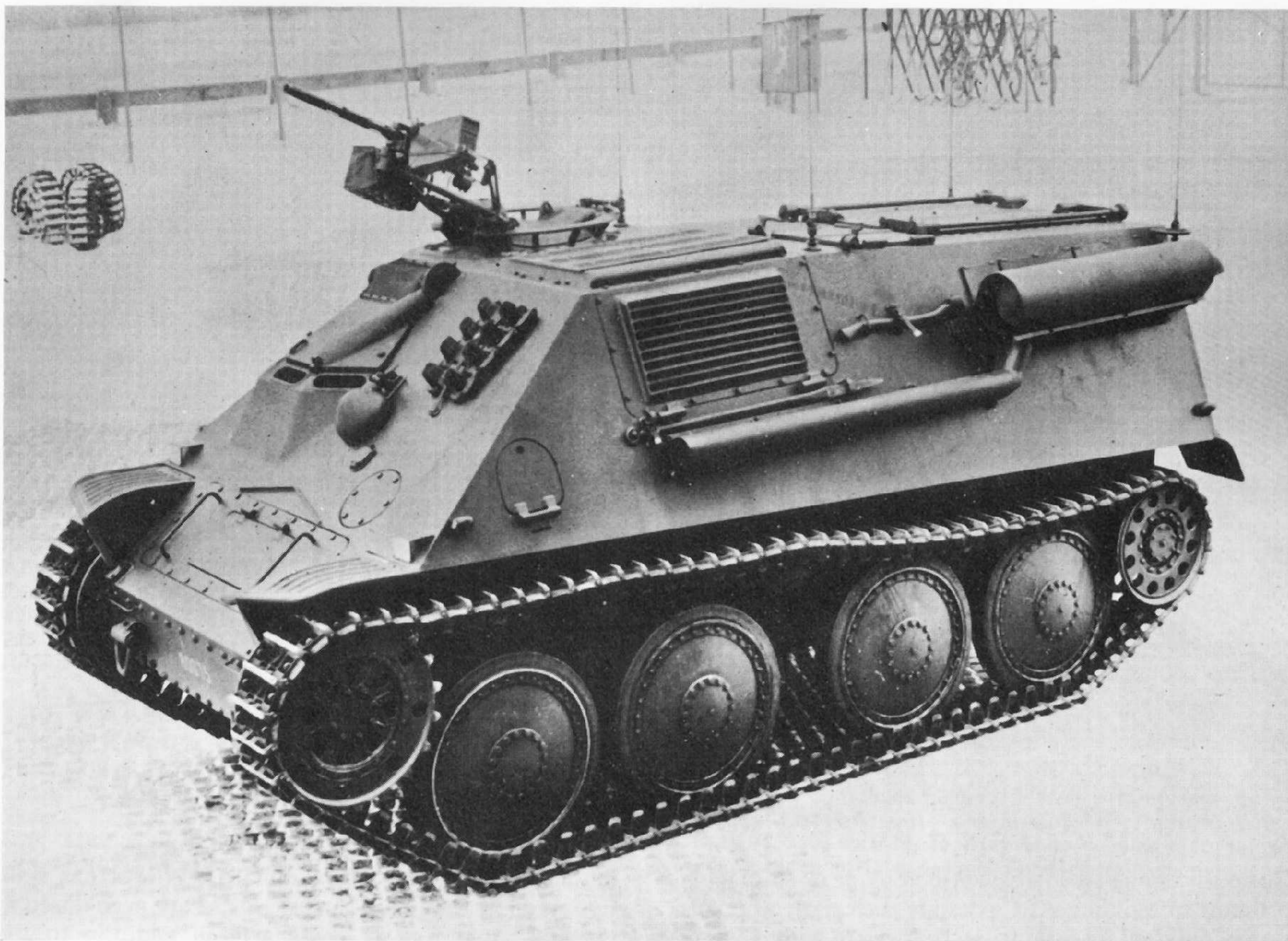
Pbv 301 was a conversion from the Strv m/41 tank, which was itself based on the Czech TNH light tank. (Pbv = Pansarbandvagn, or armoured personnel carrier).
