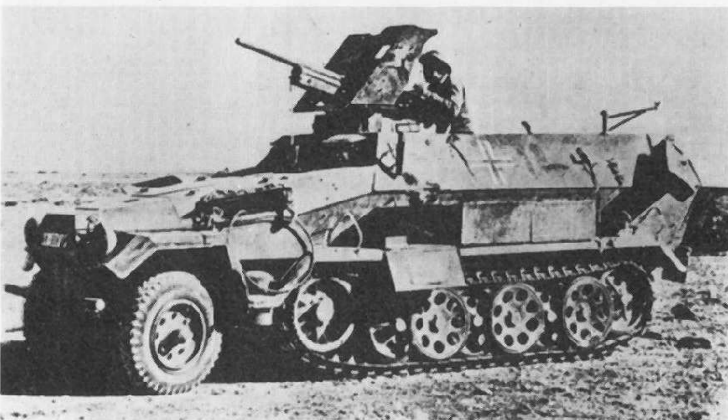
SdKfz 251/10, the variant of the German Mittlerer Schuetzenpanzerwagen for platoon leaders which mounted a 3.7cm anti-tank gun.
