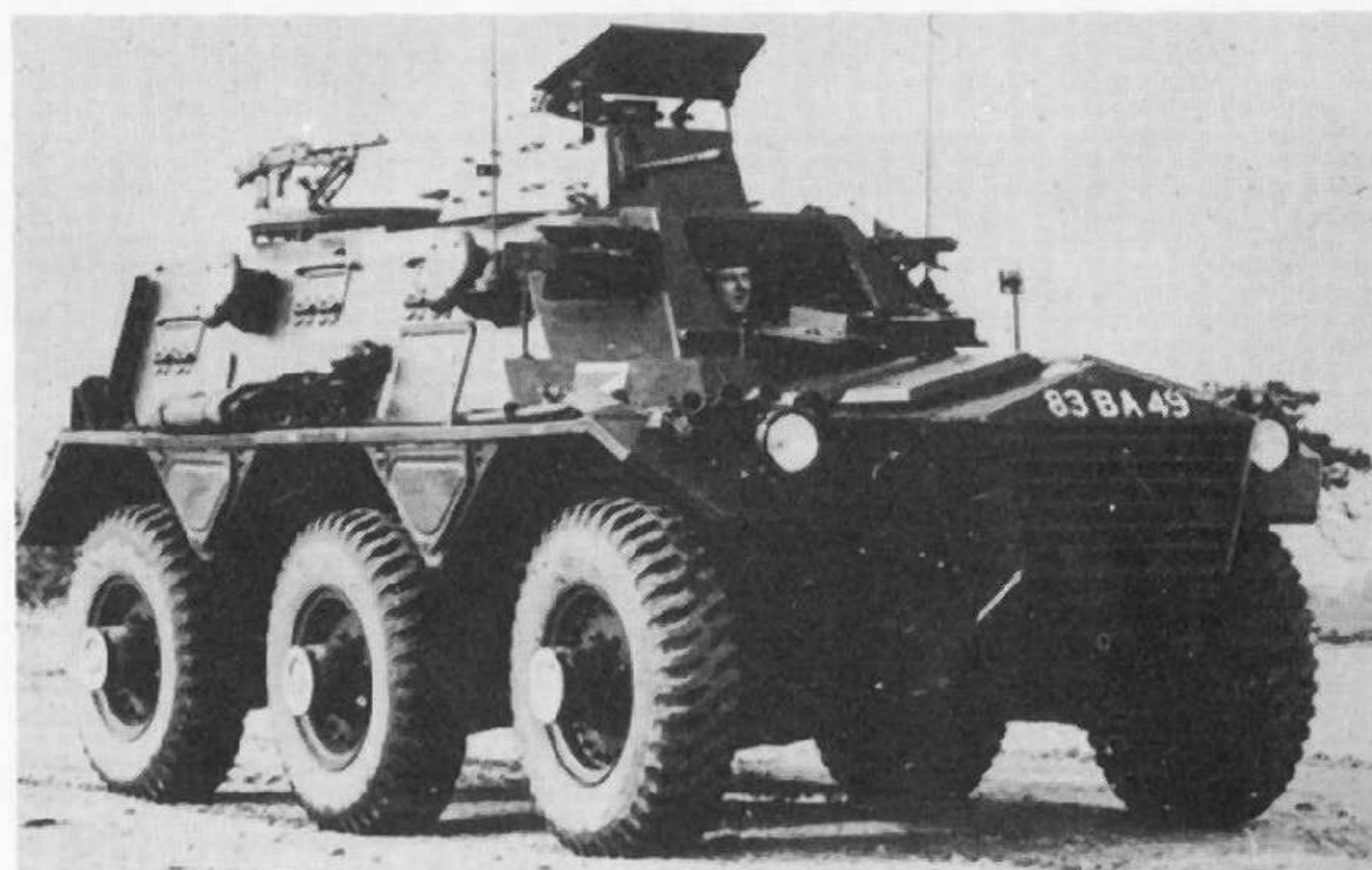
Saracen APC showing the gun turret, the open Bren, and the firing ports in the sides.
