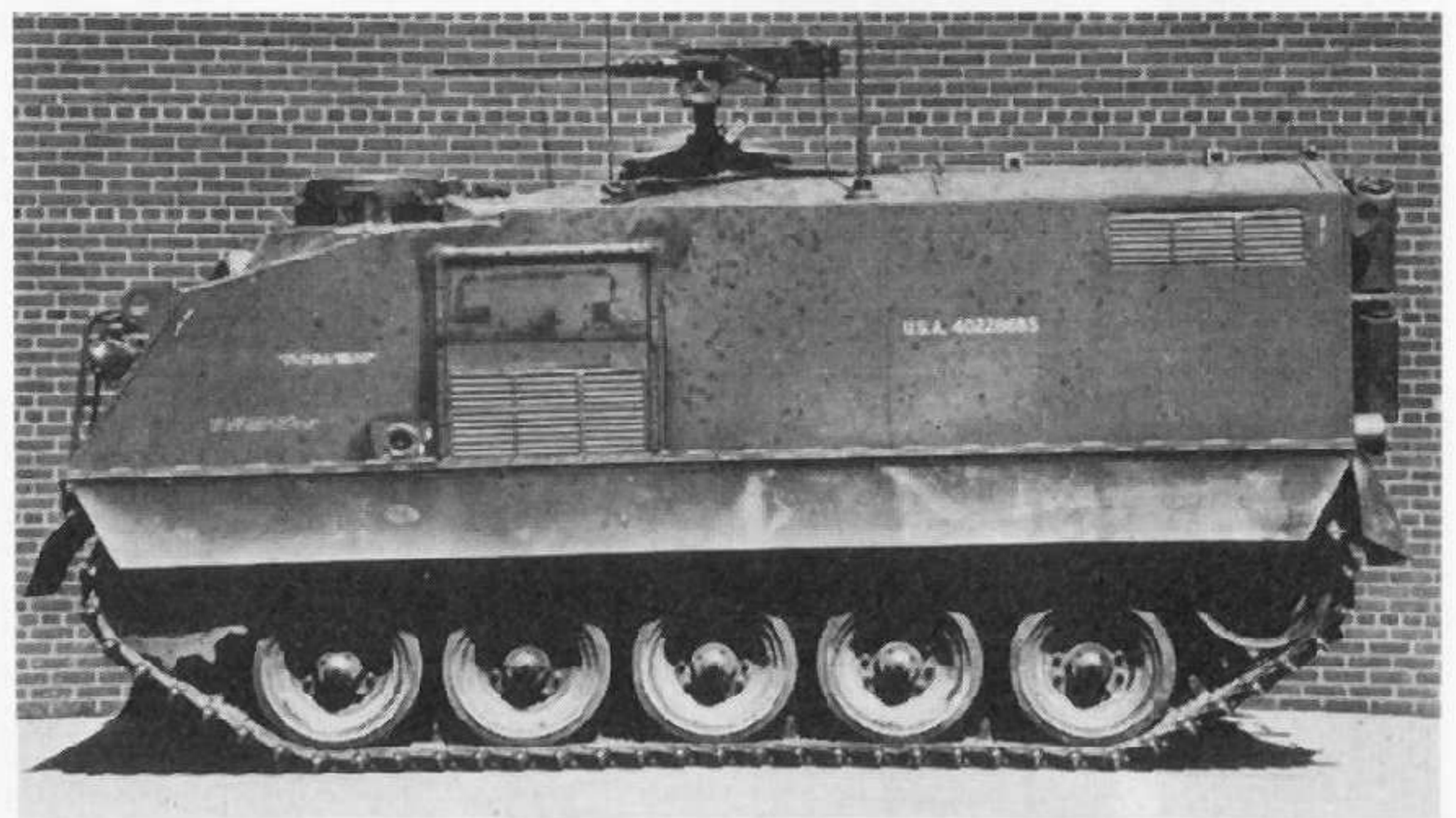
The T18 came into service in the U.S. Army in 1953 as the M75 Armoured Personnel Carrier. Note the pintle-mounted .50 cal machine-gun. (U.S. Ordnance Corps)
