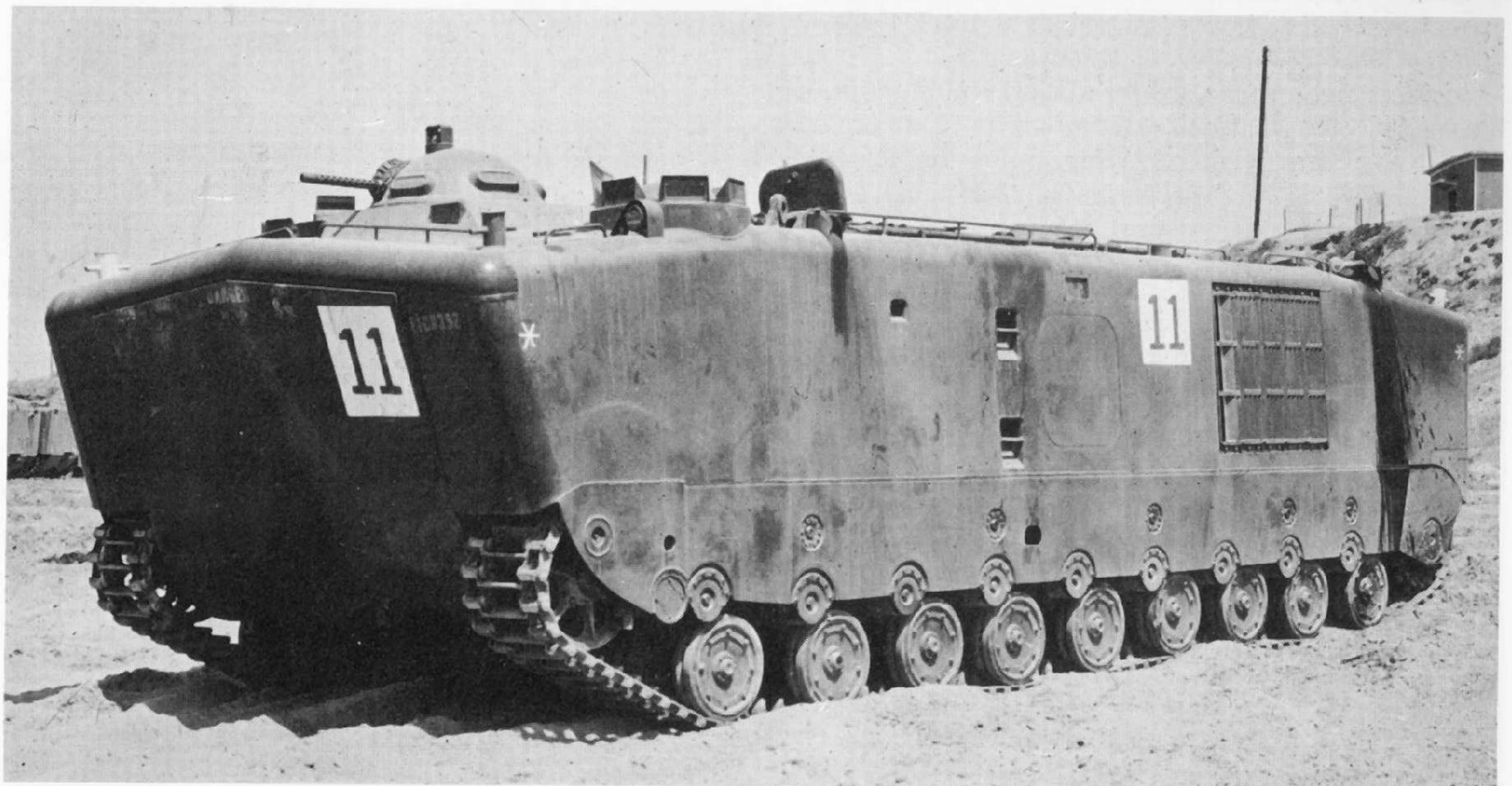
Bow view of the standard LVTP5 showing the inverted-V cut into the bow located ramp, the .30 machine-gun in the cupola, and the driver's vision device to the left of the cupola. (U.S. Marine Corps)
