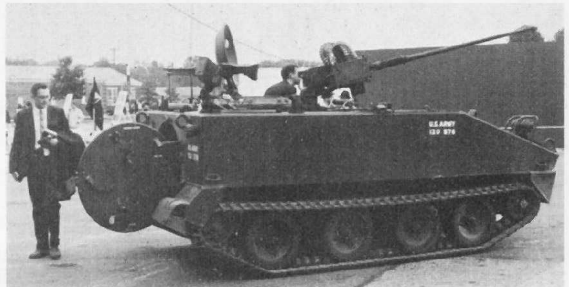
The Product Improved M113A1—no longer a battle taxi but an armoured fighting vehicle. Note the remote-controlled 20mm cannon. (FMC)
