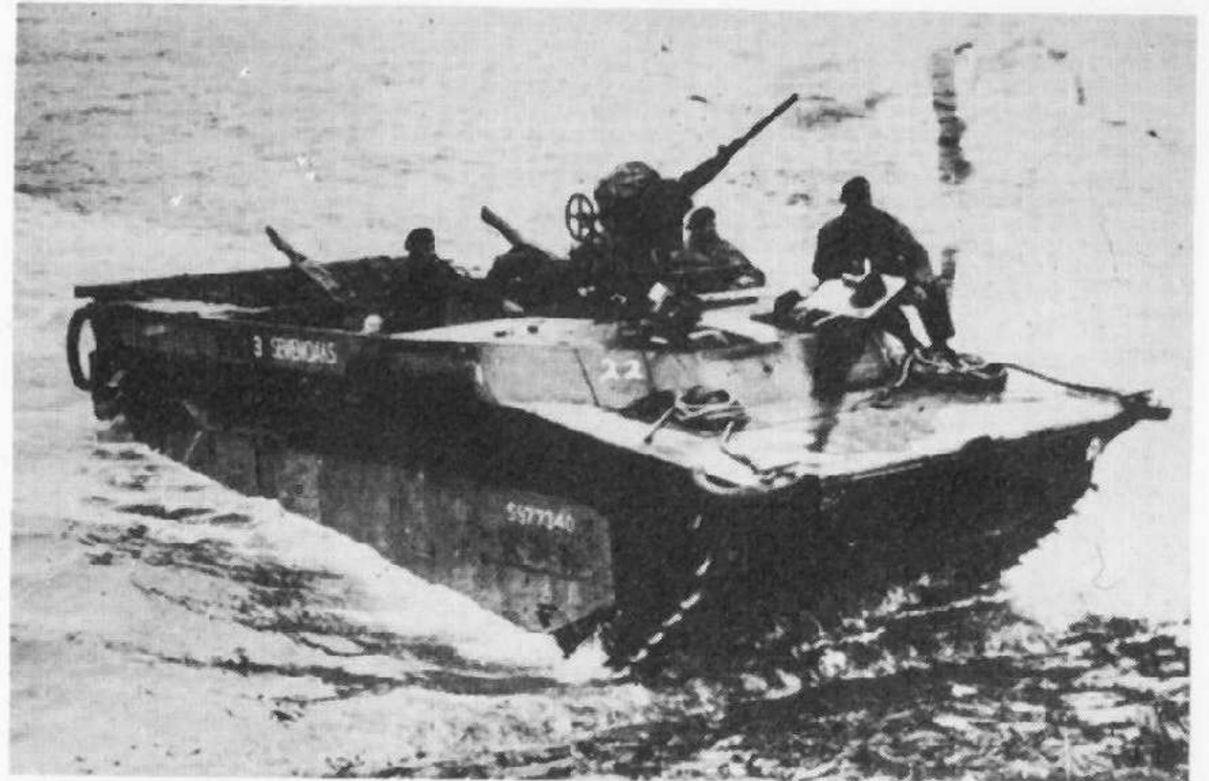
British Universal carrier, experimental version of 1948, showing the limited load space.
