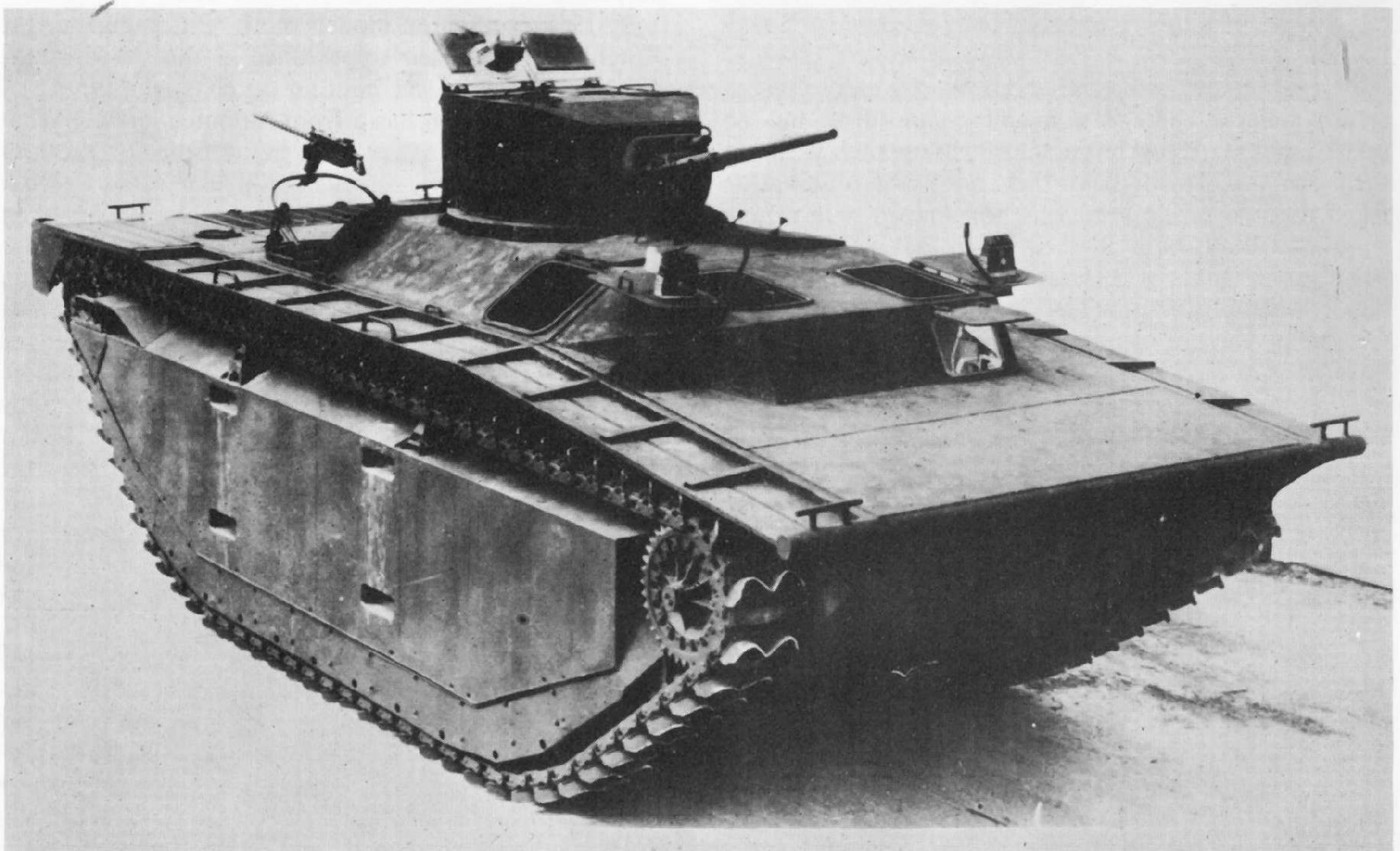
LVT(A)1: this was an armoured version of the LVT 2 with an M3 Light Tank turret mounting its 37mm gun. Note the crew hatches in the upper superstructure plate and the .30 Browning on a traversing ring.
