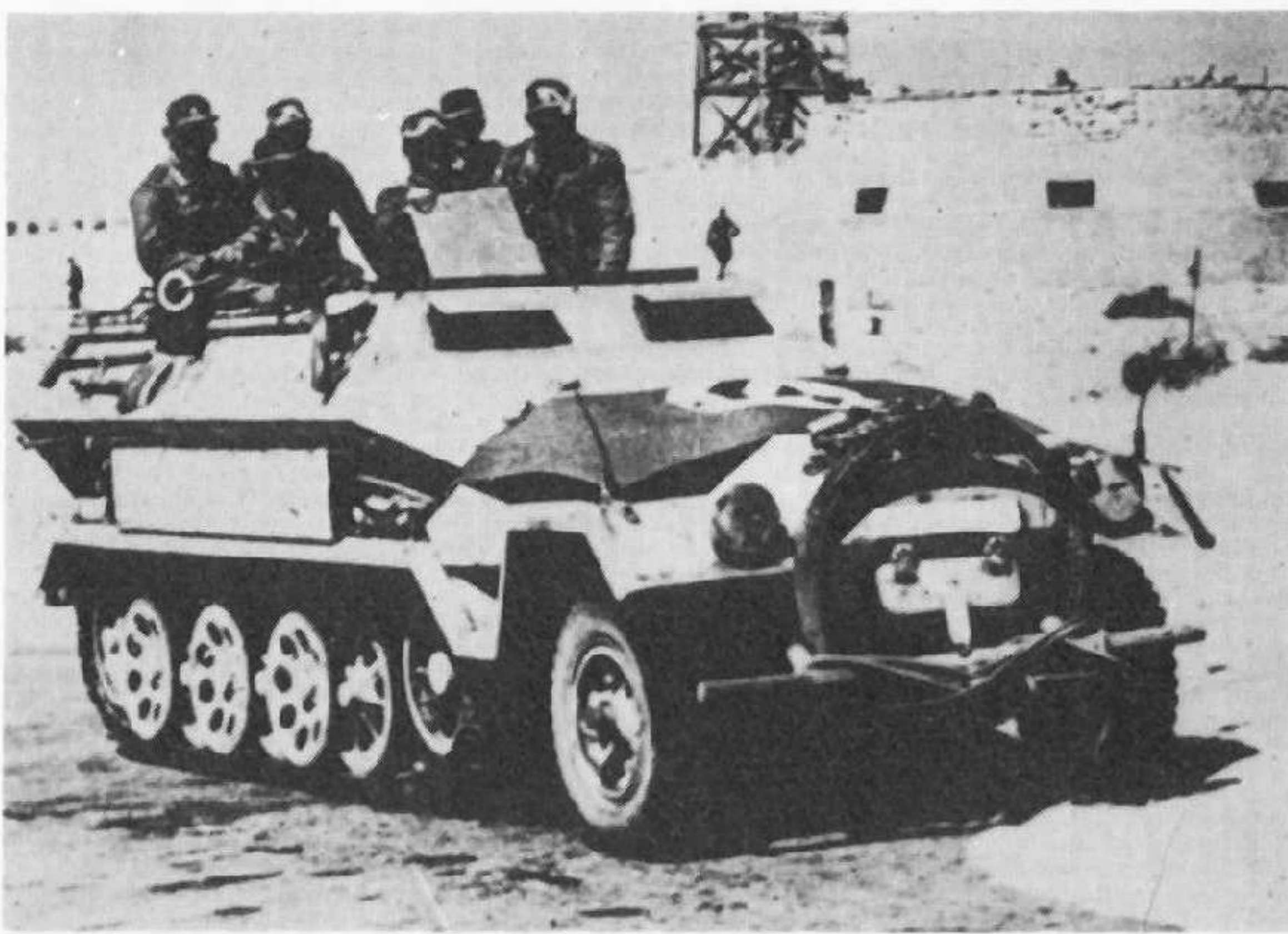
German Mittlerer Schuetzenpanzerwagen SdKfz 251/1, the basic medium armoured personnel carrier.
