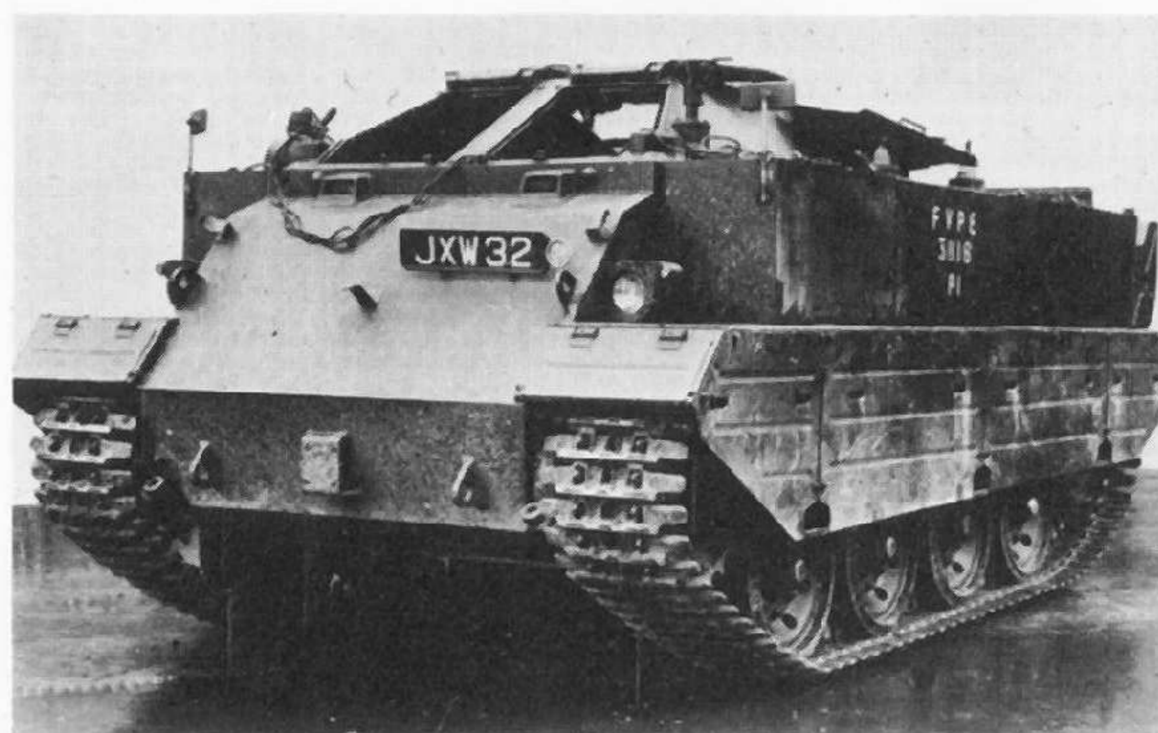
FV 401, the Cambridge carrier, appeared in prototypes only. Passengers would have had to go into action over the sides of the vehicle. (top left)
