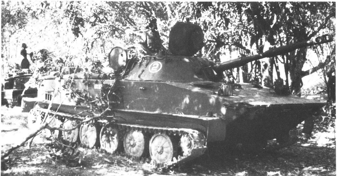
PT-76 Model 2 of the Indian Army used in the fighting in Bangladesh. (Indian Army Official Photograph).
