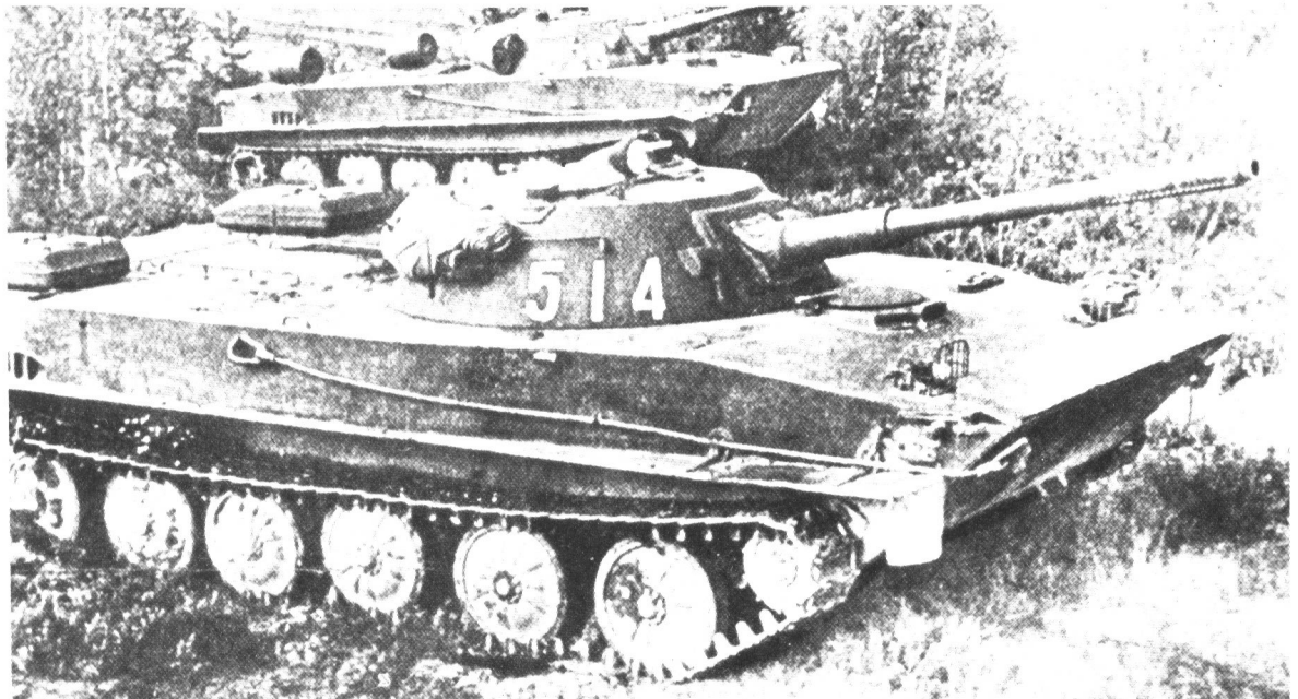
PT-76 Model 1s. Note the different type of auxiliary fuel tank carried on the rear of each hull.
