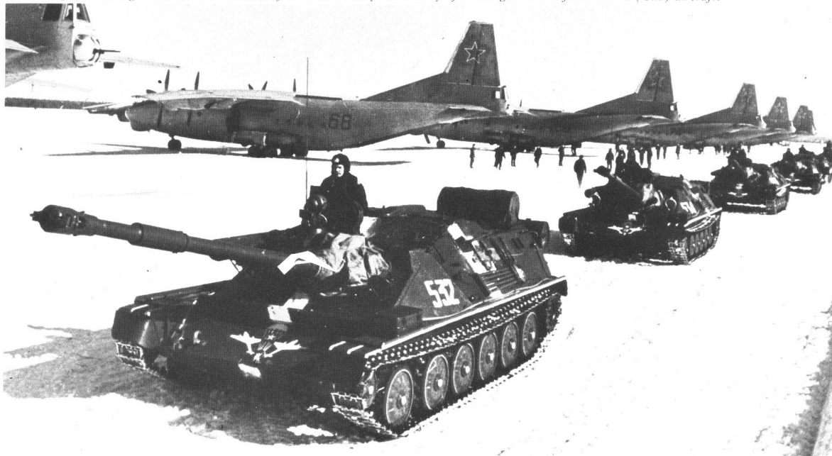
ASU-85s of the Chernigov Red Banner Division of the Soviet Army move away after being unloaded from AN-12 (Cub) aircraft.
