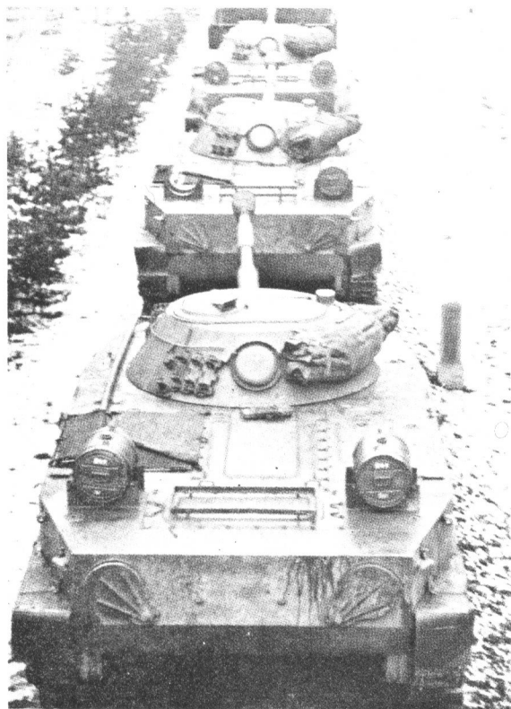
Rear view of a column of PT-76s. This clearly shows the ports at the rear and the fuel drums on the rear decking.
