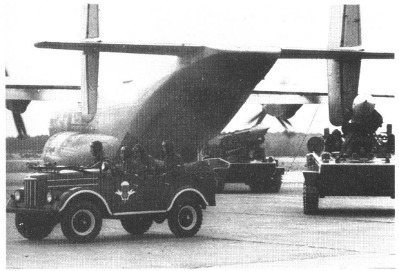
FROG-3s being unloaded from the giant Antonov AN-22 aircraft.
