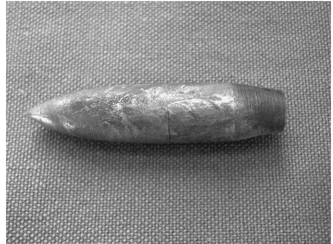
Fig. 10. Fractured core of M8 API ammunition used in PS20-2.
