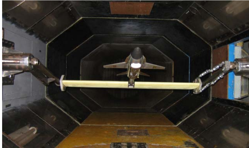
Figure 3. Pitch Damping Rig in the LSWT using the Standard Dynamic Model (SDM)
