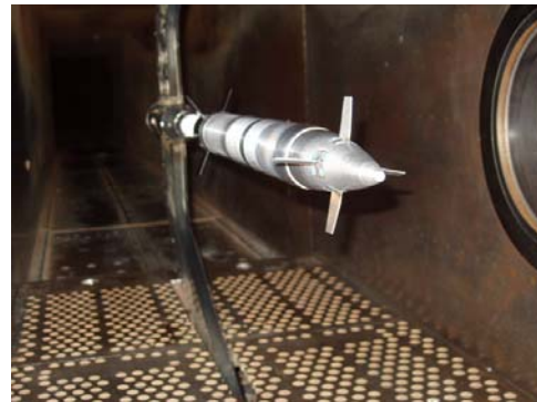
Fig.5 A model in wind tunnel
