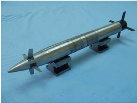
Fig.2 The geometry of model No.1 (with two pairs of canards/two pairs of wings)
