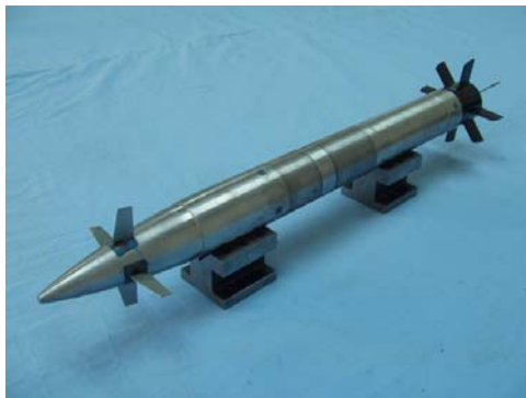
Fig.4 The geometry of model No.3 (with two pairs of canards/four pairs of wings)
