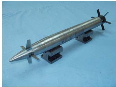
Fig.3 The geometry of model No.2 (with two pairs of canards/three pairs of wings)
