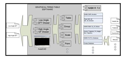
Figure 7. Graphical Firing Table Software Design Schema
