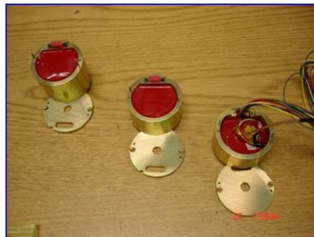
High-G Telemetry System Configuration G after encapsulation
