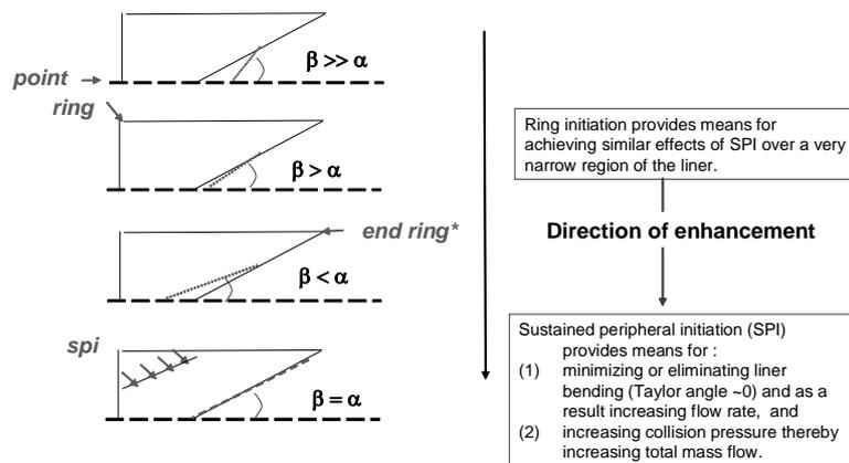
**Figure 8** Sustained peripheral initiation offers a possibility of equalling and exceeding projected performance levels of shaped charges by combining envisioned high energy futuristic explosives with today's lower energy explosives<sup>21</sup>.
