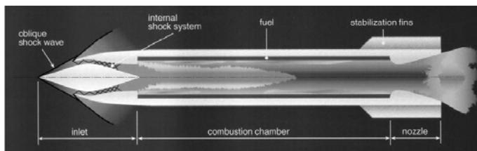
**Figure 3** Solid fuel ramjet (SOFRAM), courtesy TNO<sup>13</sup>
