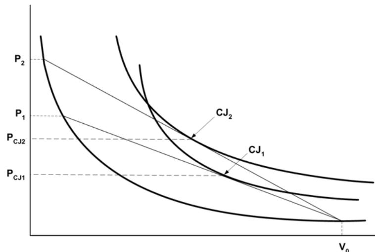
Figure 7 Differences in detonation product isentropes and C-J conditions resulting from divergent and convergent detonation
