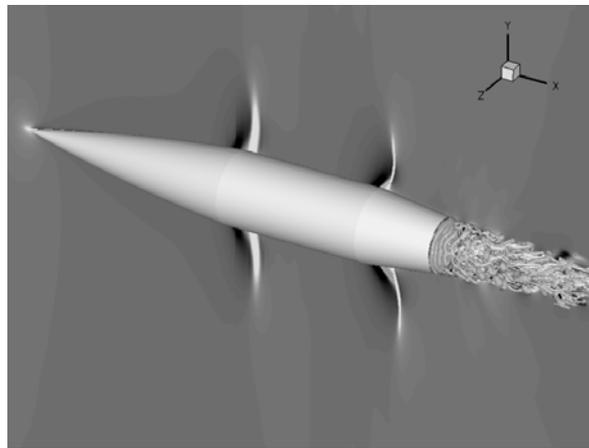
**Figure 6** Spinning projectile with boattail, ZDES computations, Mach 0.91,  $-\alpha = 2^\circ$ , pseudo-schlieren visualization, iso-contours of  $Q$  iterion<sup>16</sup>
