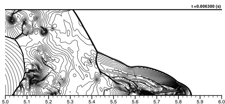
**Figures 4a, 4b** Intermediate ballistics computations, 2-D unsteady CFD of the separation process of a sabot long rod projectile<sup>14</sup>
