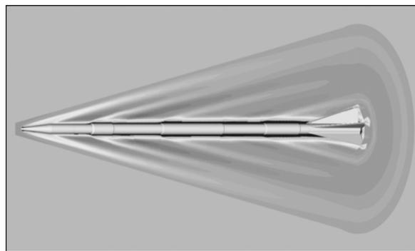
**Figure 5** APFSDS Mach number field, URANS computations, Mach 4.5<sup>17</sup>
