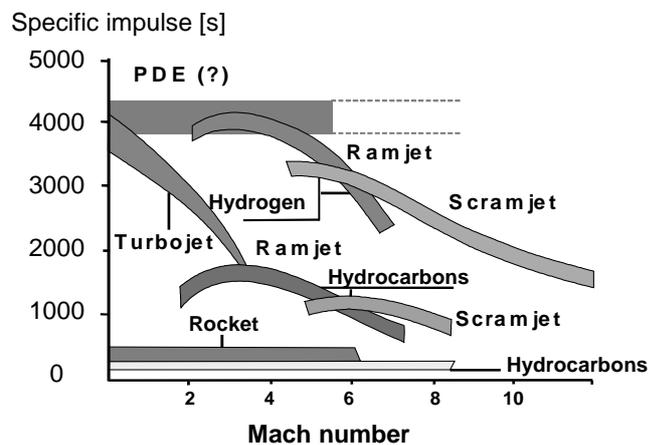
Figure 2 Specific impulse for different propulsion engines
