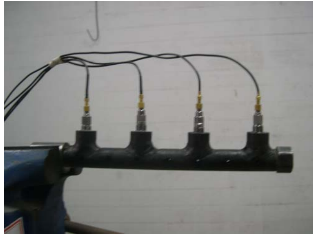
Figure 1. The experimental setup of an ignition simulator
