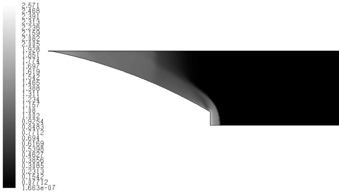
Figure 2. Oblique shock around nose of the projectile
