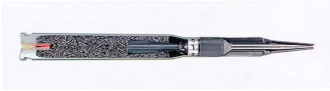
30mm, Oerlikon, APFSDS T, PMC287, V = 1405 m/s
