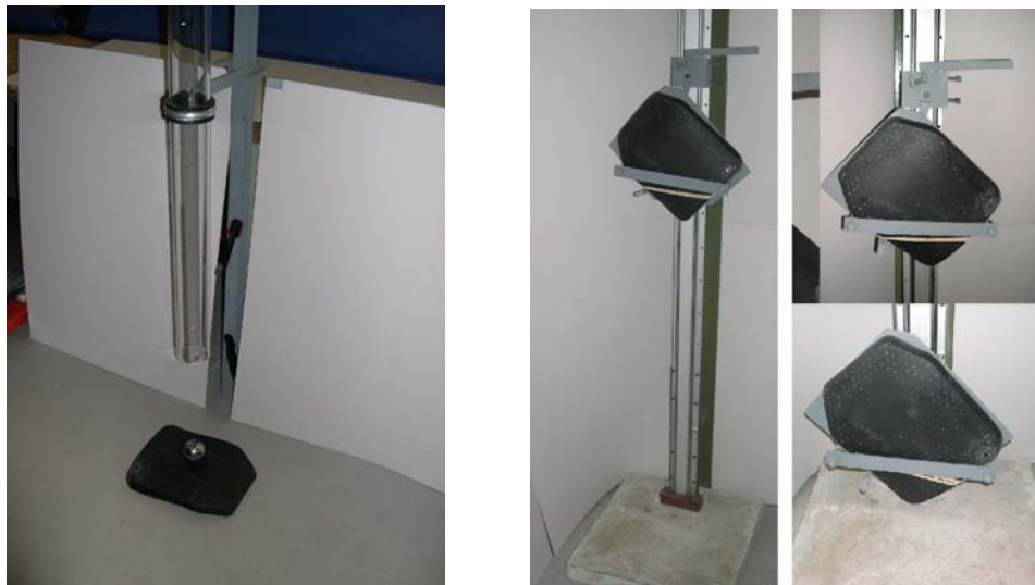
Figure 3. Left: drop test with steel ball, right: guided drop on one of the corners.
