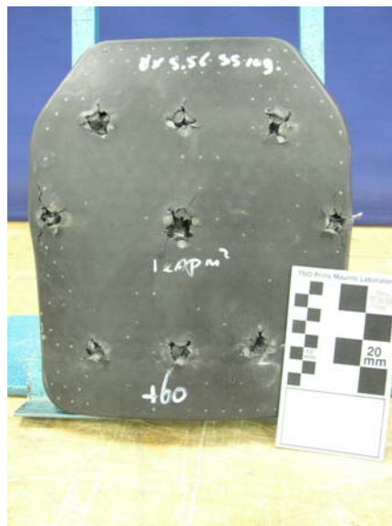
Figure 4. Picture of an insert with ceramic pellets (LIBA). The insert was hit 8 times with 5.56 mm SS109 projectiles at muzzle velocity and once with a .30-06 APM2 according to NIJ 0101.03/level IV. All impacts were stopped by the insert.
