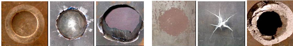
Figure 3. Typical failures of front and rear surfaces of target plates under three impact modes
