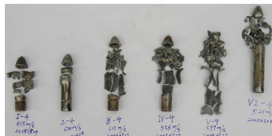
Figure 11. Broken projectiles after penetration tests under different velocities
