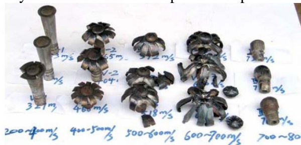
Figure 1. Variations of failure modes of projectiles under various impacts
