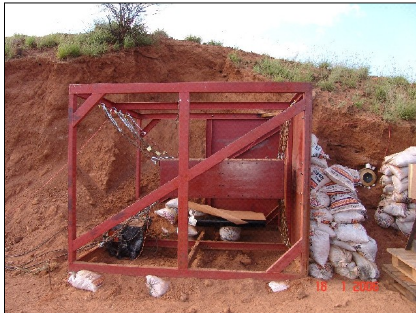
Figure 1: The set-up of the experiment, showing the FX and surrogate mine position.
