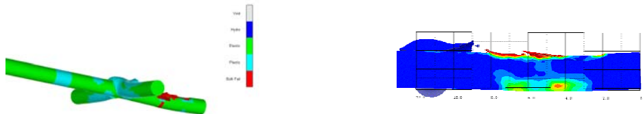
Figure 5. Simulation of one rod hitting the projectile at 600 m/s in the front of the projectile (case 2). To the left: material properties at 4.5 \mu s after hit. To the right: the frontal part of the projectile indicating the position of fracture.
