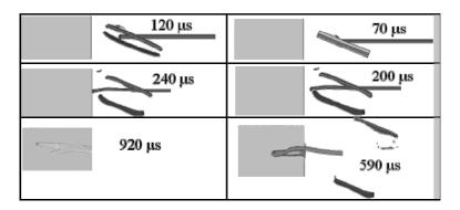
Figure 7. Projectile penetration processes into armor module cassette including witness plate
