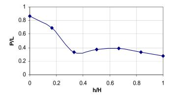
Figure 6. Penetration depth vs. impact height at ERA module
