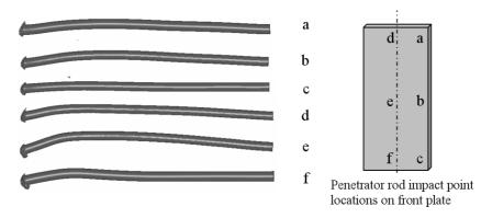
Figure 3. Projectile shapes after interaction with a reactive armor module at different locations on the front plate
