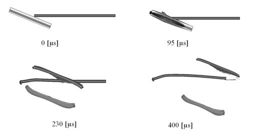
Figure 1. Projectile penetration processes into armor module cassette
