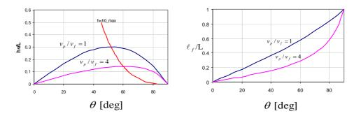
Figure 5. Minimal impact height for full interaction as a function of impact angle
