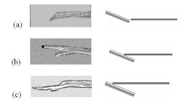
Figure 8. Crater channel shapes for different impact points after penetration into witness plate
