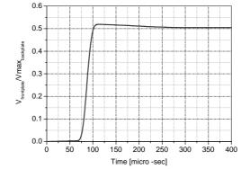
Figure 2. Reactive armor front and back plate velocity ratio
