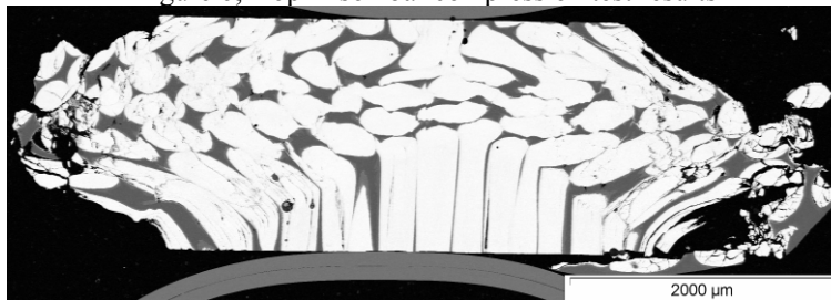
Figure 7; Cross-section of dynamic compression testpiece
