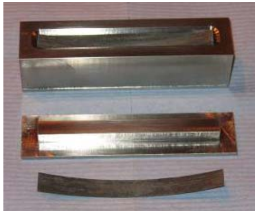
Figure 1; HIP block, piston, layer of wire preform
