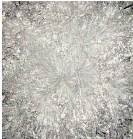
Fig. 8. Central damage pattern in the last layer of glass, viewed through the polycarbonate.
