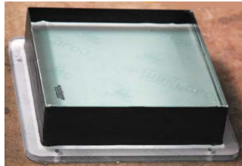
Fig. 1. Seven layer glass target. Glass outside dimensions are 304 \times 285 mm. The seven-layer target contained 76 mm of glass on 12.7 mm of polycarbonate.
