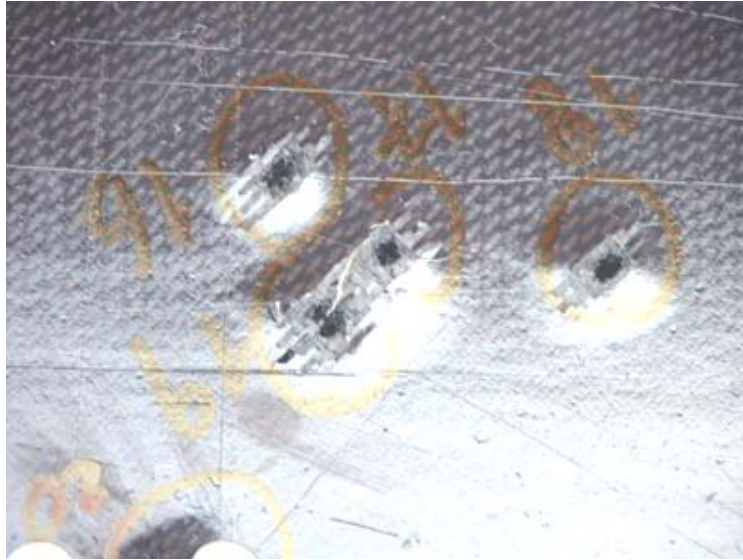
PHOTO 2: Front Panel after the Test: Detail of impacts.
