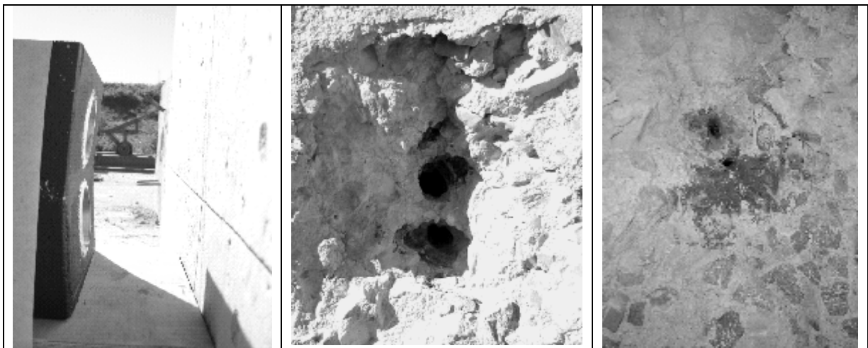
Figure 6. Setup and Entry and Exit cavities in the target for the sub-calibre firings
