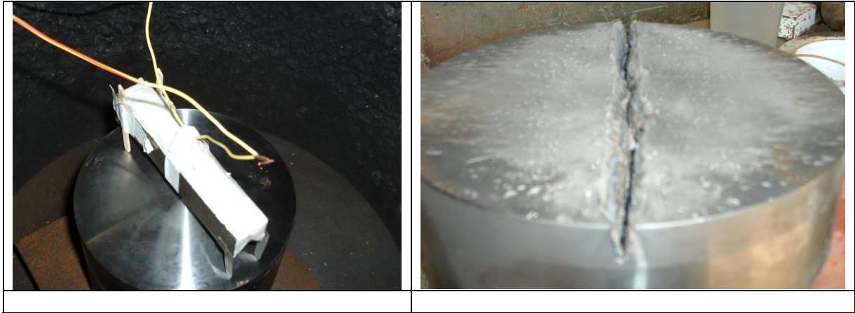
Figure 4. Initial LSC penetration testing.
