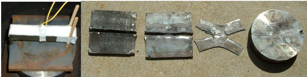
Figure 6. Initial LSC target buffering plate penetration test setup and results
