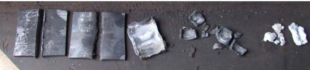
Figure 10. Test results of PBXN-9: 2 buffer plates (left), steel body (center left), end cap pieces (center right) unreacted explosive (right).
