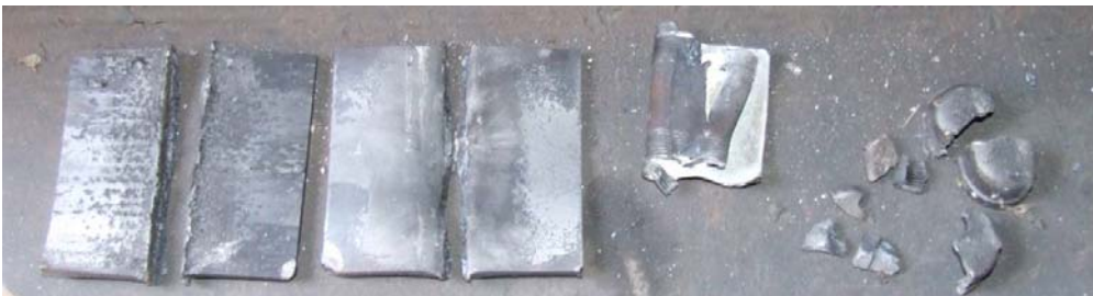
Figure 9. Test result of Comp A3: 2 buffer plates (left), steel body (center), end cap pieces (left).
