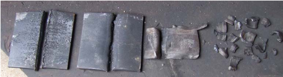
Figure 8. Test result of Comp B4: 2 buffer plates (left), steel body (center), end cap pieces (left).
