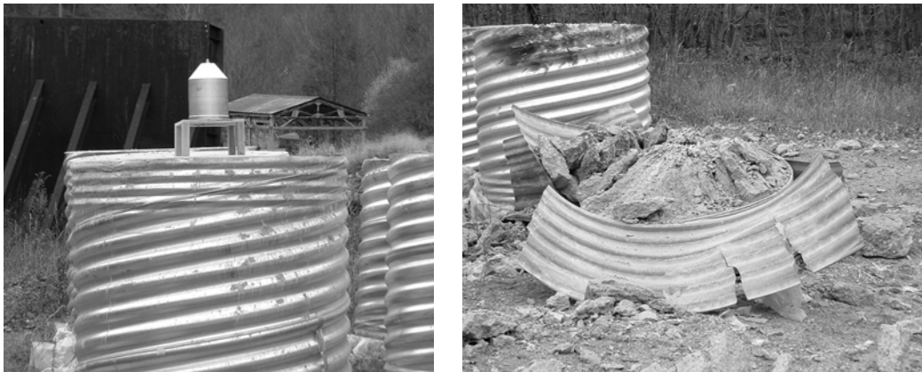
Figure 5. Bam Bam warhead tested against a 1.5m (five foot) diameter concrete culvert.
