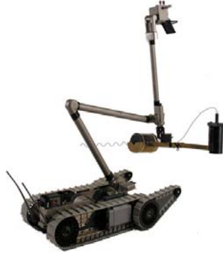
Figure 7 Robot with remote emplacement assembly
