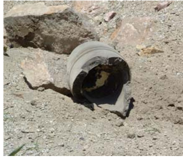
Figure 5 Large base fragment with unreacted Composition B
