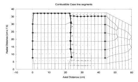
The same initial configuration was used for the next example, but igniter gas was released inside **both** modules. Only vertices defining line segments were moved. The grid and velocity vectors are depicted in the figure below. The calculation could not be continued beyond the stage shown, due to zero/negative cell volumes occurring next to the second module. An algorithm for the sympathetic movement of vertices not defining line segments is obviously needed.
