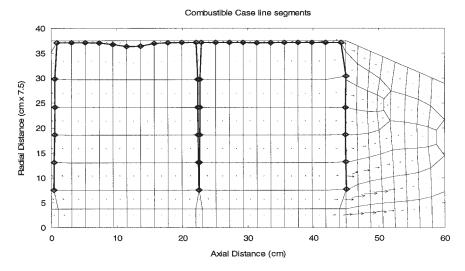
A basic algorithm for moving these vertices is to reposition them at the average position of their direct neighbours. Several iteration cycles are needed. Vertices on the outer boundaries must obviously remain on these boundaries. The result for this simple scheme,
