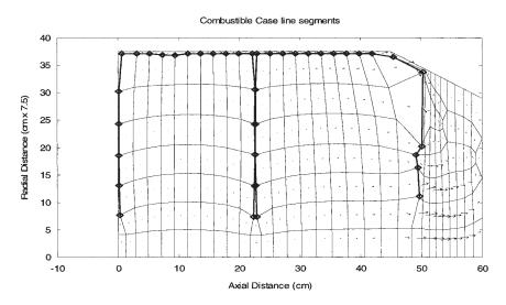
The previous problem was repeated for a much longer period of time and the improved mesh movement algorithm was used. The result appears above. The movement of front wall of the second module appears to be unstable, with one very large face and several small faces. This instability can be attributed to the lack of material strength as well as a rupture mechanism in the present model. The algorithm for sympathetic movement appears to function satisfactory.
