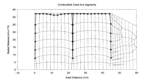
In response to grid problems encountered as different calculations were run for longer times, the grid movement algorithm was continually refined. The end result is an algorithm were the position of a vertex (not defining a line segment) is calculated as a weighted average of the positions of its direct and indirect neighbours. The weights are modified when problems like small interior angles or short cell sides occur.
