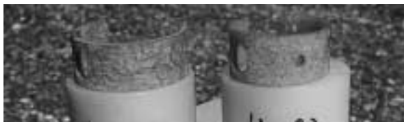
Figure 5: Pre-treated transparent JA2 by a plasma arc (0,8 kJ left and 1,5 kJ right).
