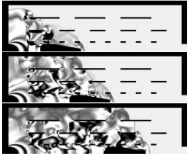
Figure 7. Muzzle muffler pressure distribution at bullet exit.
