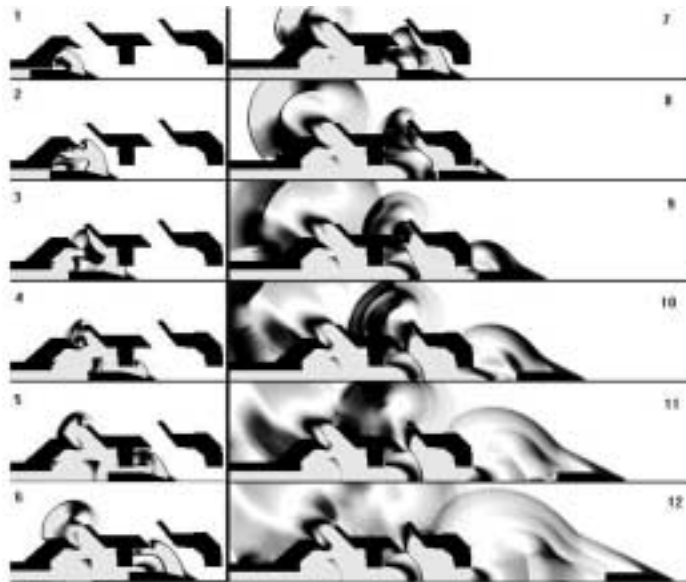
Figure 5. Pressure distribution in the intermediate ballistics period for a gun with muzzle break.
