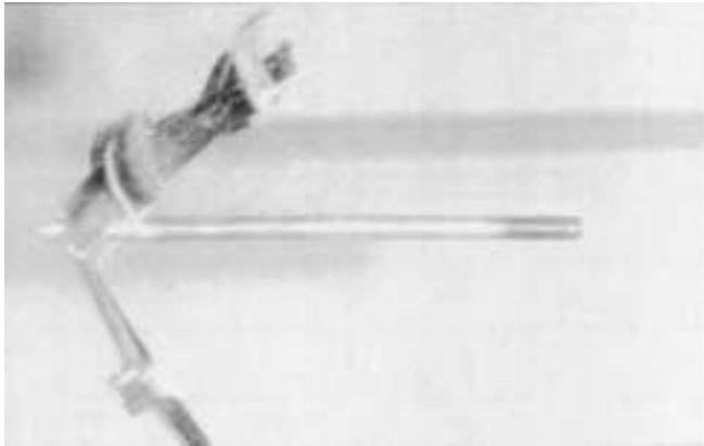
Figure 1. “The Lonely Jacket”. The problem Sabot-parts discarding from the steel jacket; tungsten core and fins are left behind (disassembled) due to insufficient joint properties of core/jacket.
