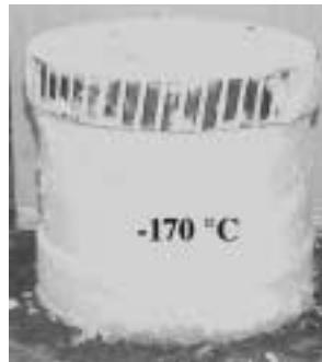
Figure 11: Shrinking of the rotating band on a sample.
