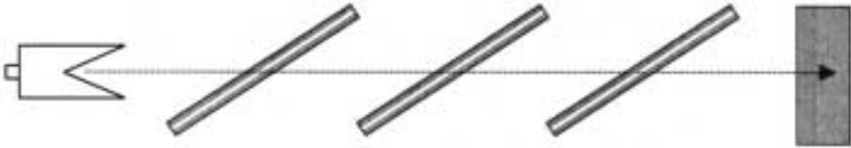
Figure 1: A typical ballistic experiment setup of a single shaped charge warhead against a multi-cassette target.
