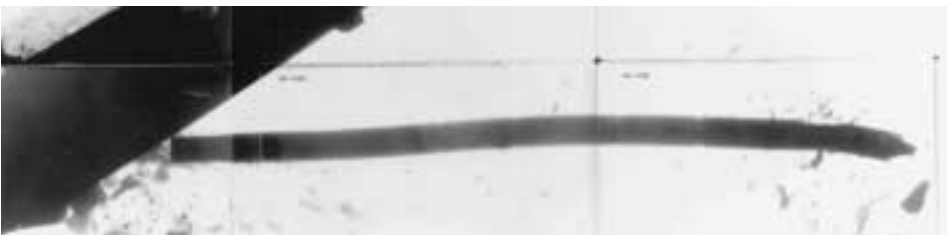
Figure 6: Full scale penetrator with steel jacket. (X-ray by GR/FS264, Thun Switzerland) Impact angle 60 NATO, impact velocity 1510 m/s, perforation.
