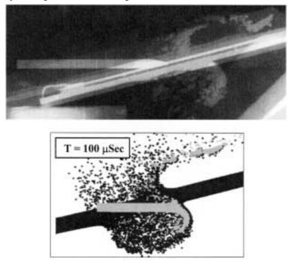
Figure 4: Test A – Top: X-ray Photo (0 and 100 sec after impact). Bottom: Simulation (0 and 100 sec impact).
