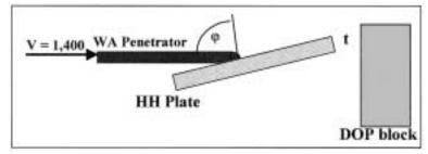
Figure 1. The Experimental Set-up.
