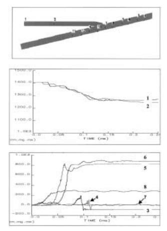
Figure 5: Test B – Axial Velocity Histories. Top: Tracer points Center: Rod tracer points 1 and 2 Bottom: Target tracer points 3–8
