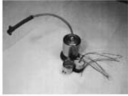
Figure 5: Complete measurement unit (above) and interior parts-embedded amplifier and fitting rings (below). With its steel casings the whole unit weighs about 330 g and has a dimension of 40 mm x 40 mm.
