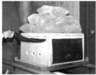
FIGURE 9: Wooden cage for the exclusion of disturbing gases and detonation flash.
