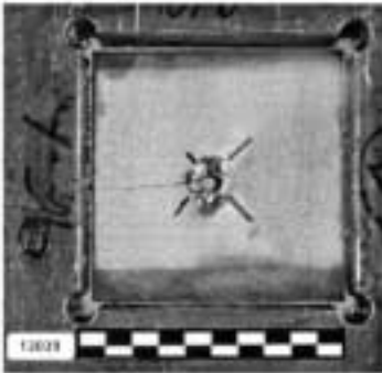
Figure 6: Impact side (left) and back side (right) of a Cermet 3 specimen in a DOP configuration.
