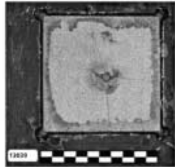
Figure 6: Impact side (left) and back side (right) of a Cermet 3 specimen in a DOP configuration.
