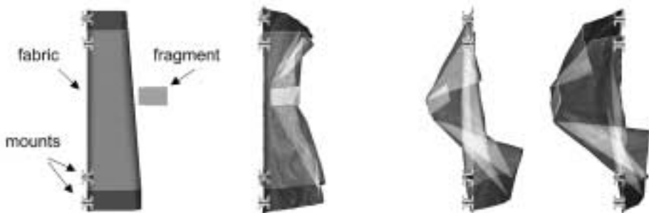
Figure 4: Simulated response of fabric for full-scale fragment impact test.
