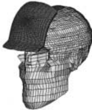
Figure 7: DGA head model with delaminating part of helmet.
