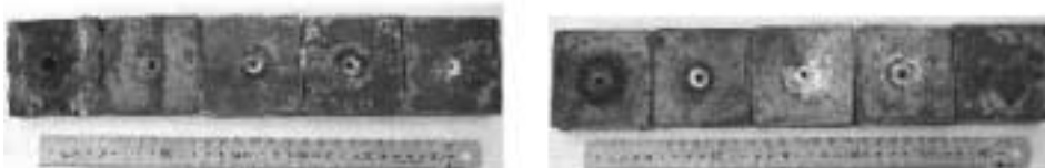
(a) Top faces (b) Bottom faces Figure 5: Photographs of penetrated steel blocks in No. 6 experiment.
