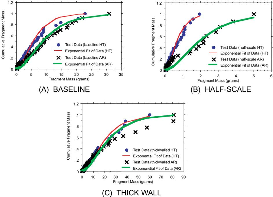
Figure 4. Cumulative fragment mass distributions heat-treated and as-received materials.
