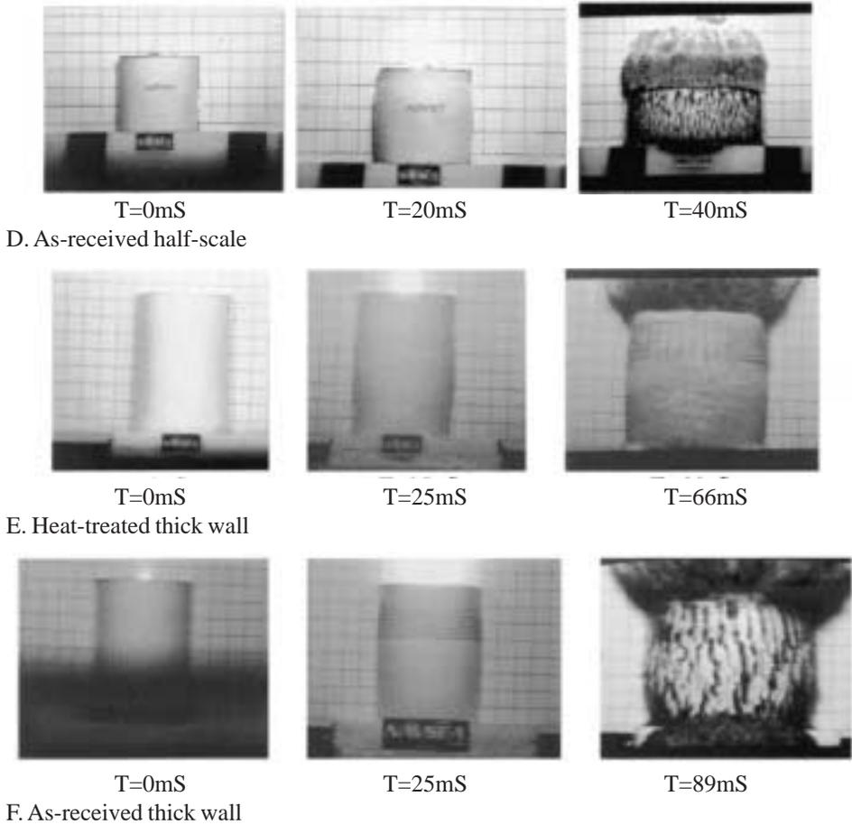
Figure 3. High-speed photos of case expansion.
