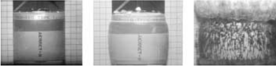
Figure 1: A Cylinder Expanding due to the Detonation of an Explosive Charge.
