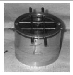
Figure 4: Subscale test warhead.
