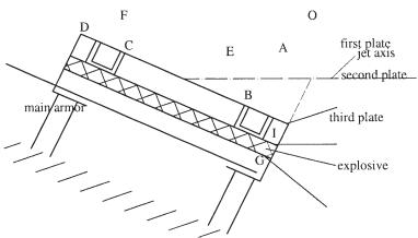
Fig. 1. Simple configure of reactive armor
