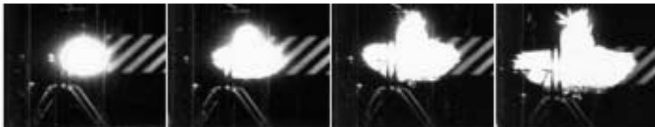
Figure 2. Hycam frames illustrating expansion of the fireball and fragment interruption of fire ball edge.
